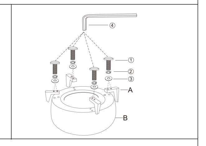
Assemble the leg to the Ottoman body with Washer, split-ring washer and Bolt.
