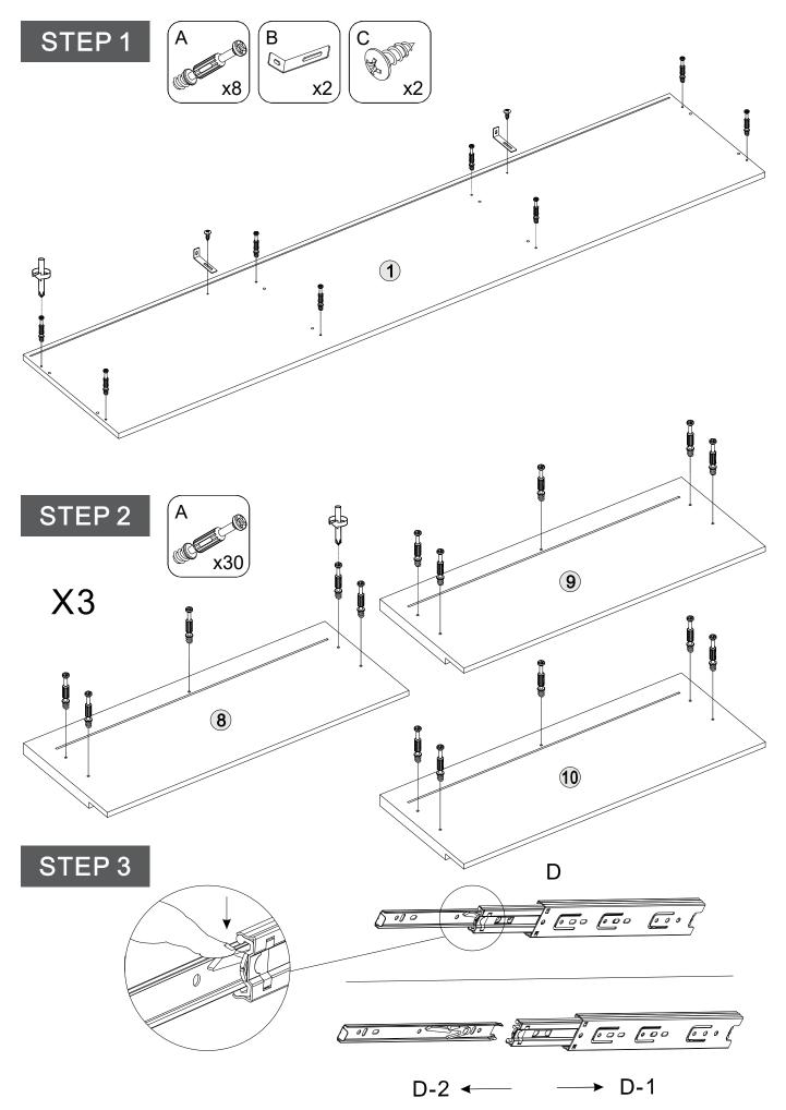
• Press the button and extend the slide slowly. Then separate it with the release latch. Repeat these steps for the other slides.
