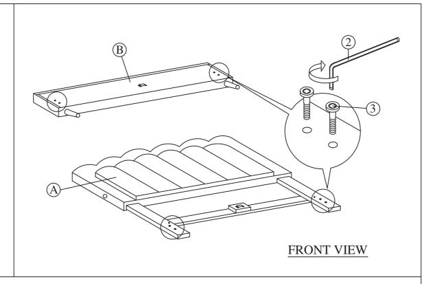
Attach the JCBB Bolt (3) to the headboard leg (E/F) and footboard (B) by using Allen Wrench (2).
