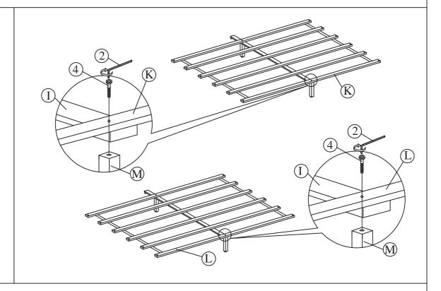
Attach the support legs (M) to the center rail (I) and slats (K/L) by using Bolt (4) with Allen Wrench (2).
