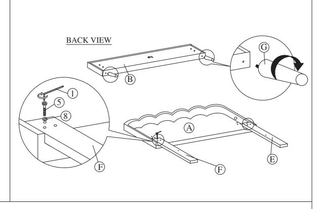
Attach the headboard legs (E/F) to headboard (A) by using Bolt (5), Spring Washer (8) with Allen Wrench (1). Attach the footboard legs (G) with footboard (B) as shown. **FULLY TIGHTEN THE BOLT.**
