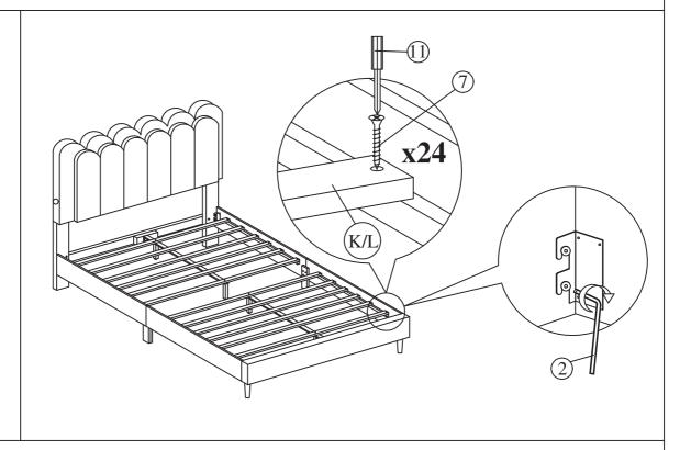
Tighten the 4 Corner with Allen Wrench (2). Install the bed slats to side rail. Tighten the slats with CSK screw. The distance of the slats should be sufficient to obtain desirable bed stability.
