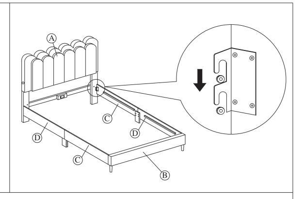
Attach side rail (C/D) to headboard (A) and footboard (B) by pushing the bracket down to fit it.
