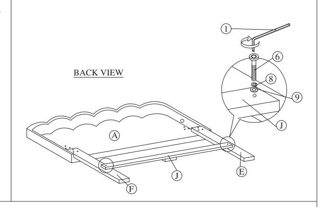
Attach the headboard leg support wood (J) to headboard legs (E/F) by using Bolt (6), Spring Washer (8), Flat Washer (9) with Allen Wrench (1).
