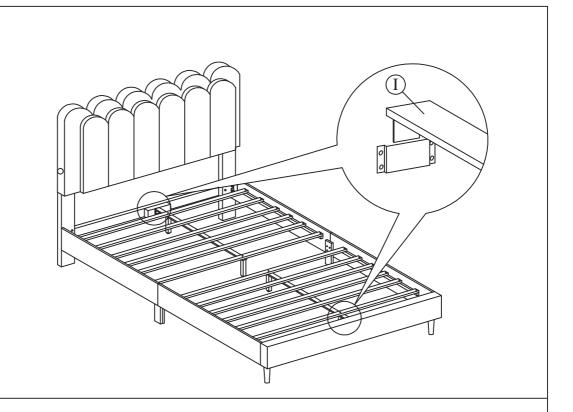
Slide the center rail (I) to the headboard leg support wood (J) and footboard (B).
