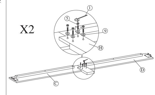
Attach the side rail leg (H) to the side rail (C/D) by using Bolt (5), Flat Washer (9) with Allen Wrench (1).
