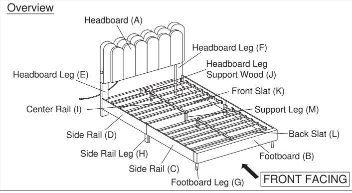
This Bed has multiple parts and may require up to 30 minutes to assemble. To give you an overview of the Bed parts, the above picture is provided to help you put the various parts into perspective. Please read through the instructions below to familiarise yourself with the parts and steps before assembly.
