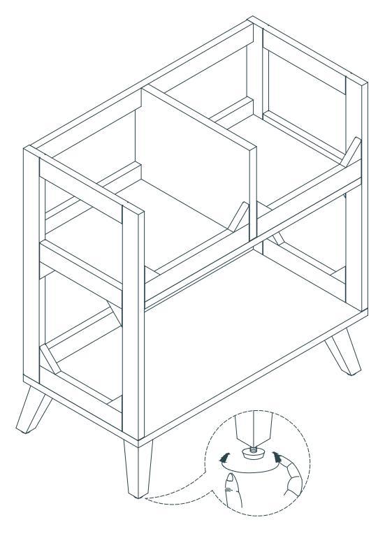
Note: It is important to adjust levelers once fully assembled and upright. Extend adjustable leveler until it's firmly in contact with the floor. If relocating, adjust leveler as needed until it's firmly in contact with the floor in new location.
