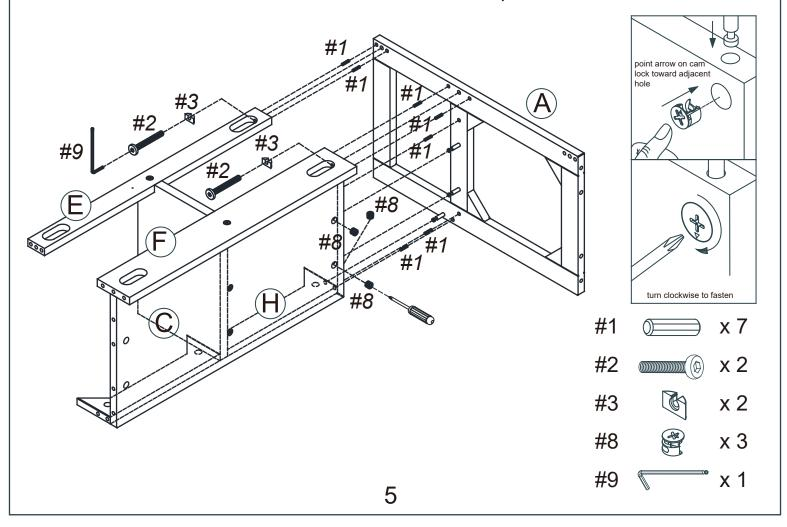
Step 5. Attach right frame (part B) and back bottom rail (part I) to assembled unit (parts A, B, C, E, F & H) using wood dowels (part #1), cam locks (part #8), long bolts (part #2), crescent washers (part #3), allen wrench (part #9) and phillips head screwdriver.
