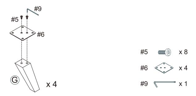
Step 8. Attach assembed legs (part G) to bottom panel (part D) using short bolts (part #5) and allen wrench (part #9).
