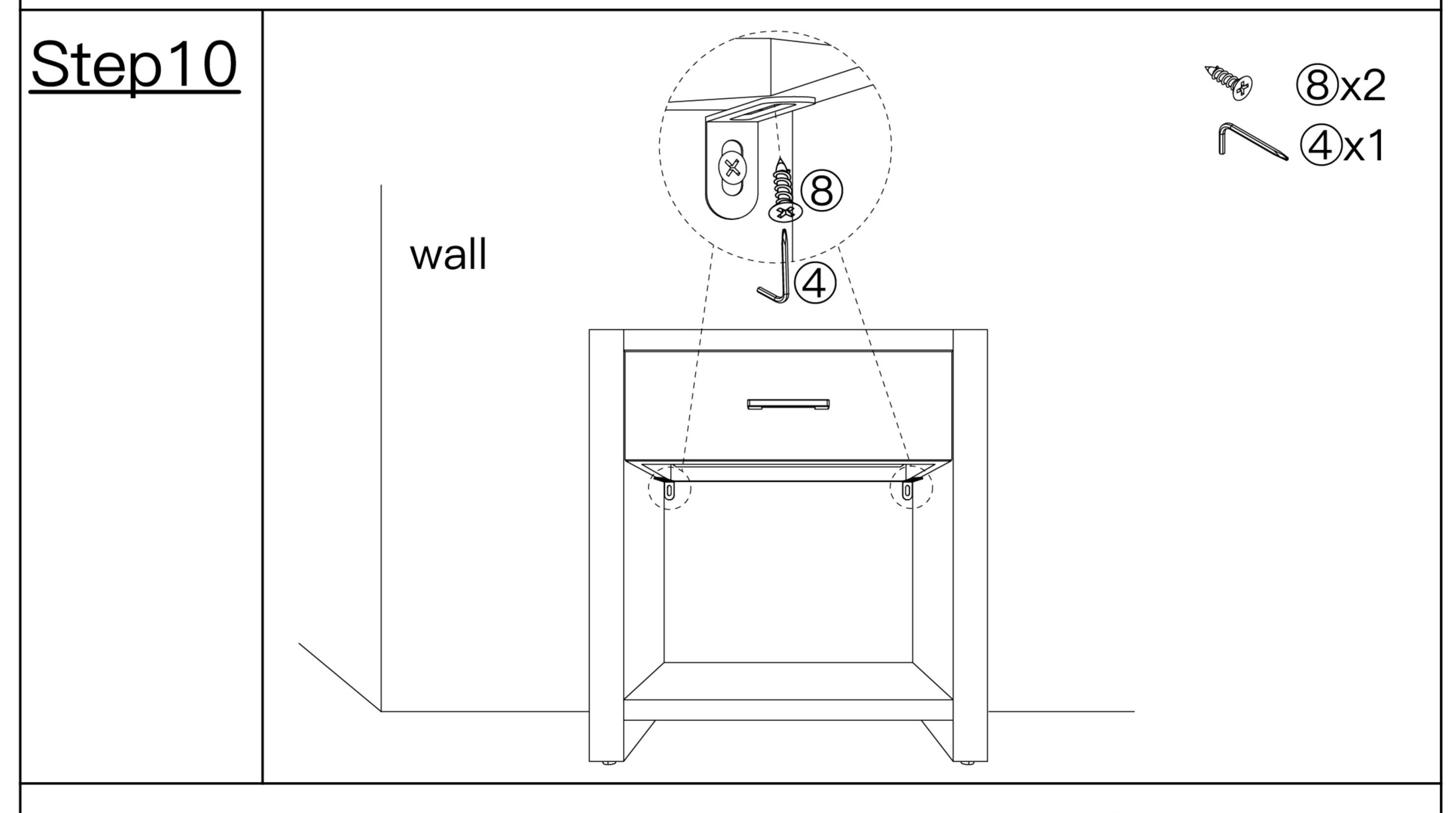
Attach the short side of Anti-Tip anchoring strap (5) to the bottom of table top (A) with short screw(8).
