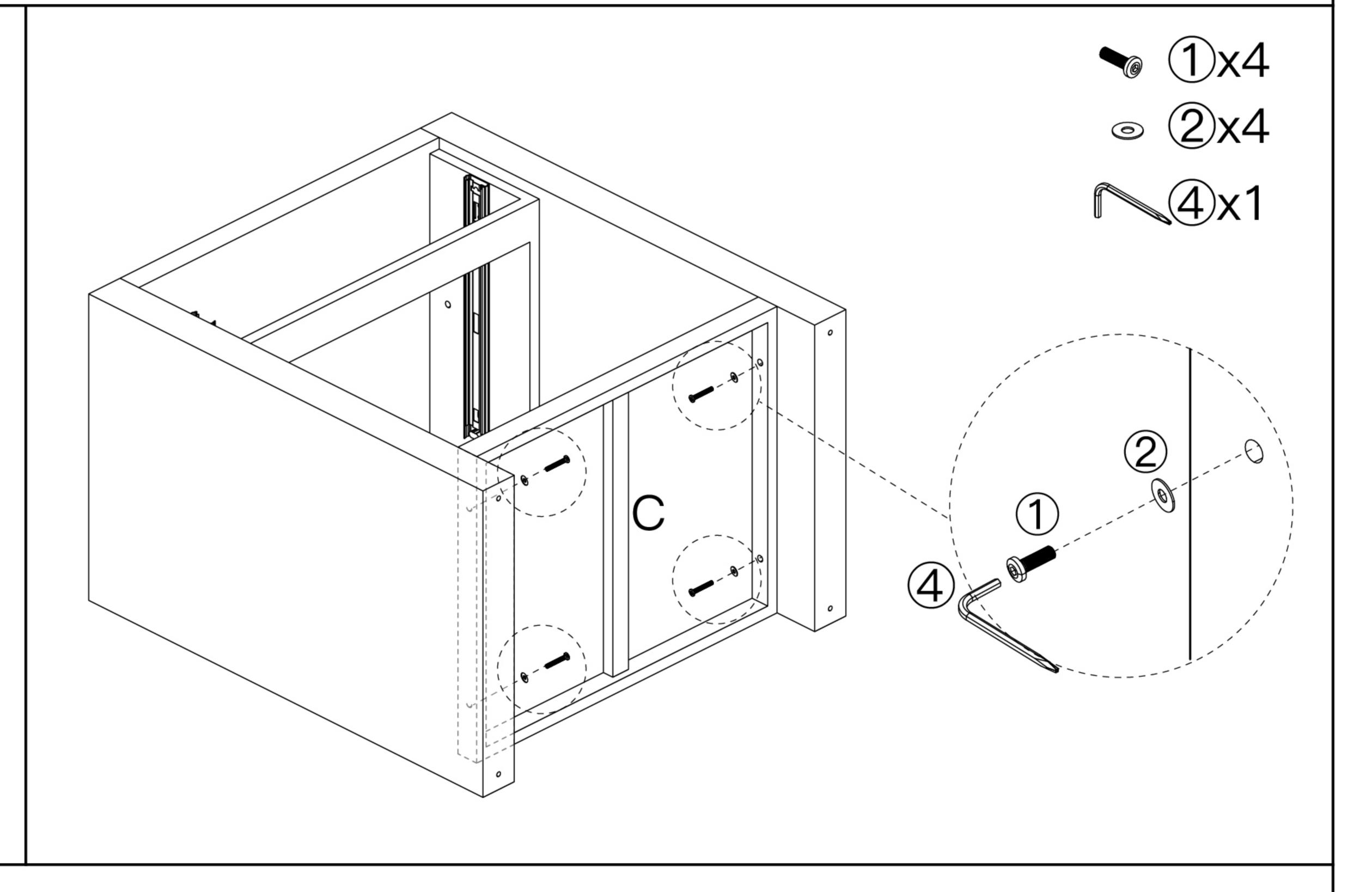
Attach shelf board (C) to side board(B) with long bolt( $\bigcirc$ 1) and flat washer ( $\bigcirc$ 2).
