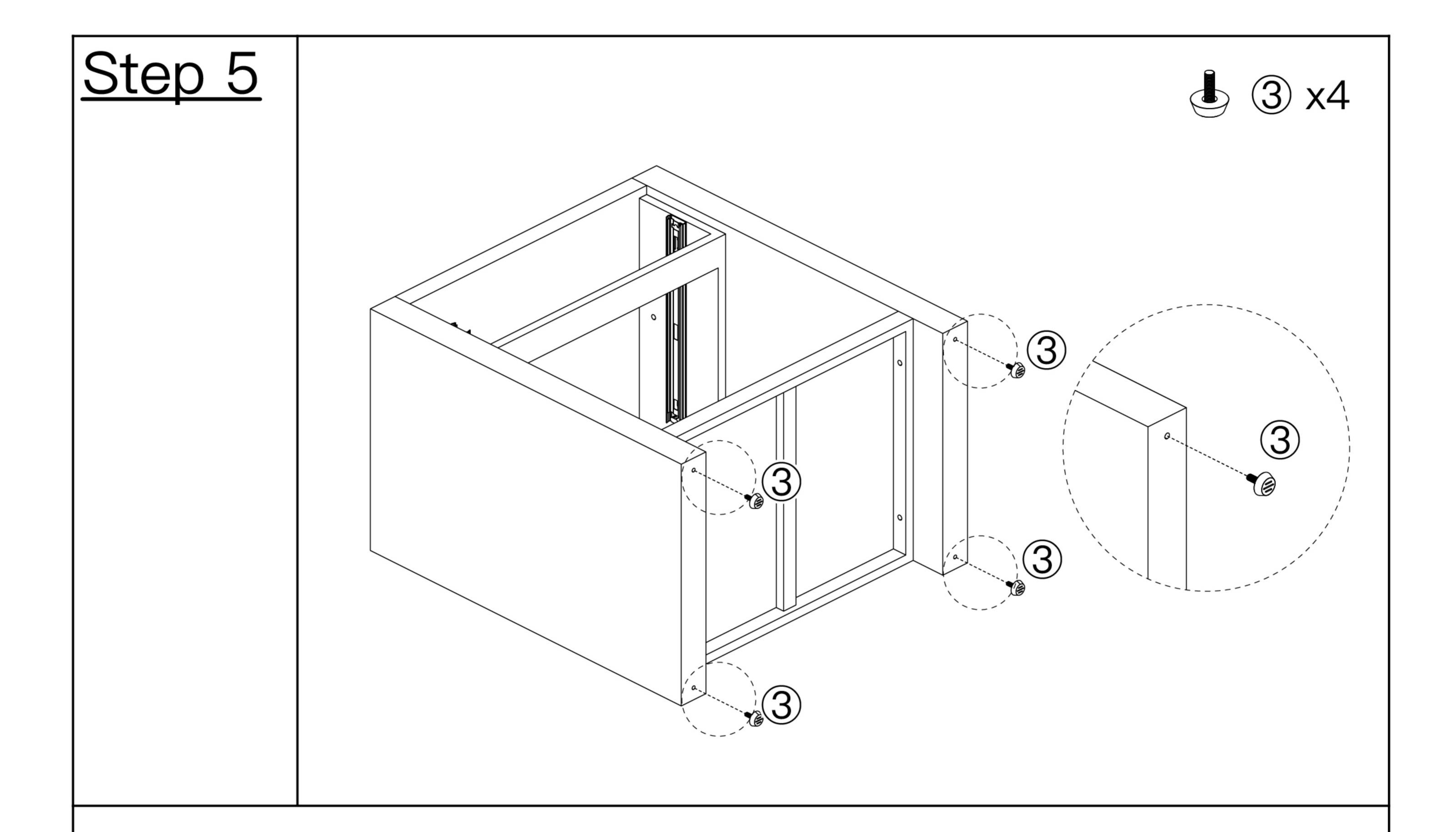
Screw adjustable leveling glide(3) to side board(B).
