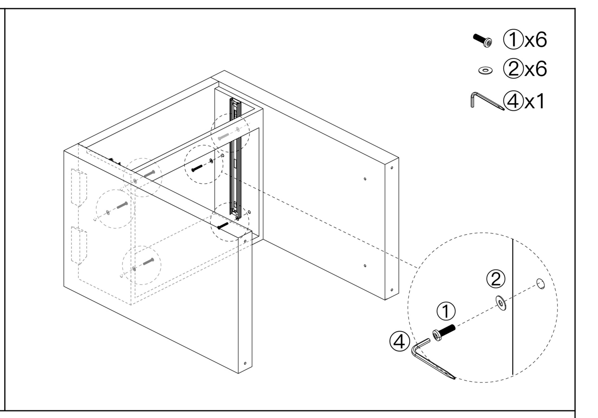
Attach table top(A) to side board(B) with long bolt( $\bigcirc$ 1) and flat washer ( $\bigcirc$ 2).
