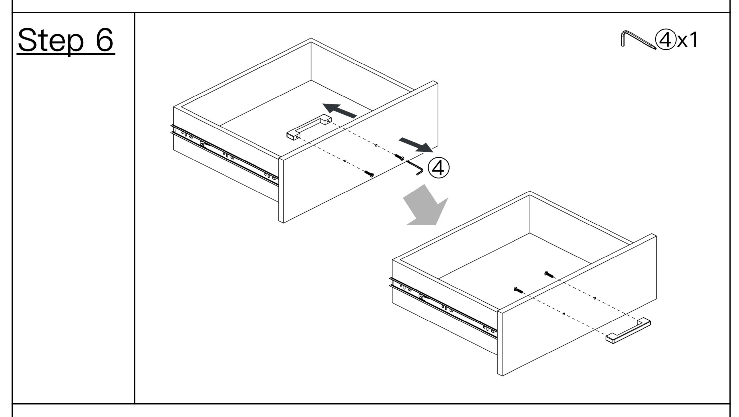
Unscrew handle from inside of the drawer, then fix it on the outside of the drawer.
