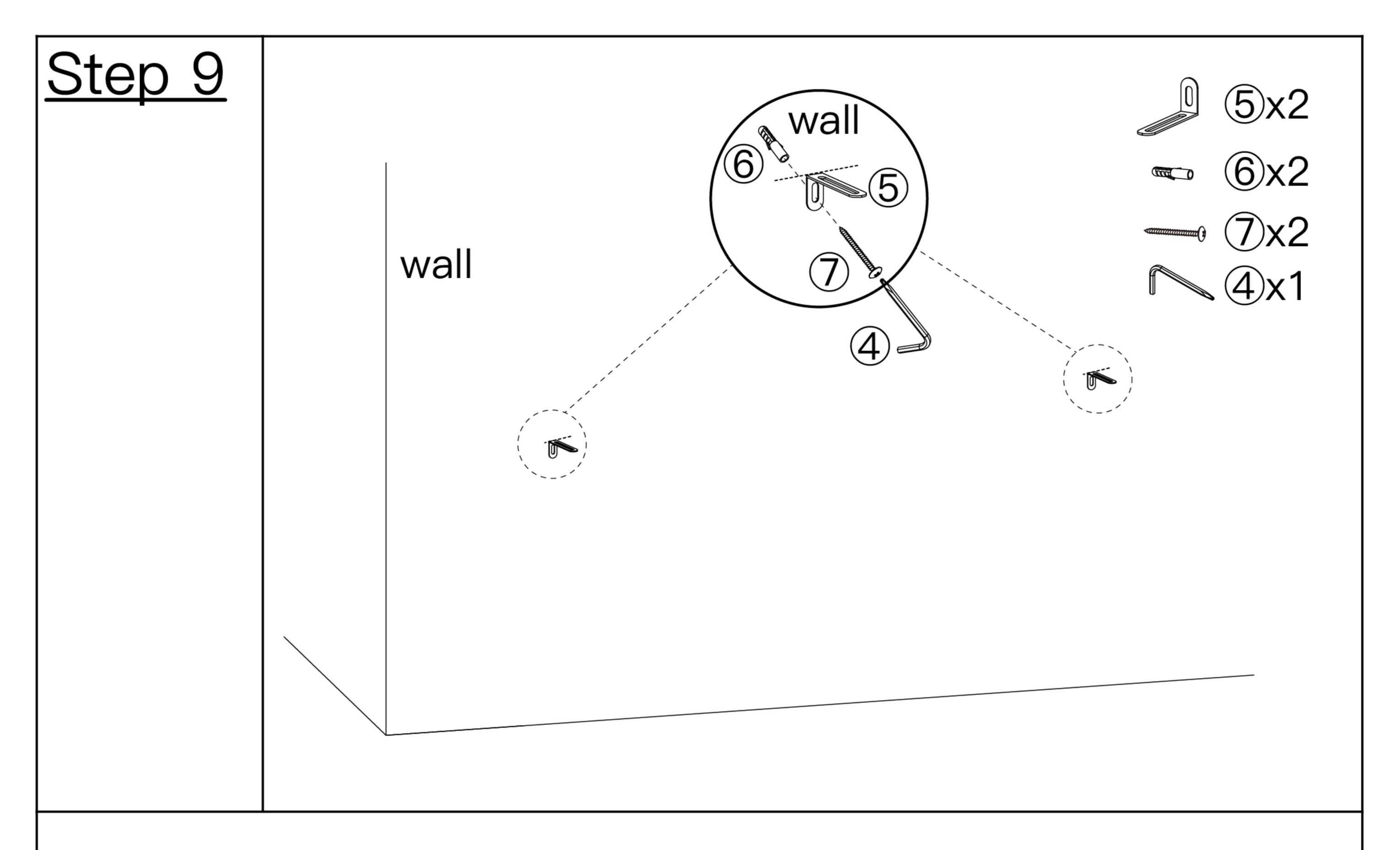
Drill holes on the wall in marking position, insert expansion plugs(6)into the holes, align with the expansion plugs (6),install the short side of Anti-Tip anchoring strap (5) on the wall with long screw(7).
