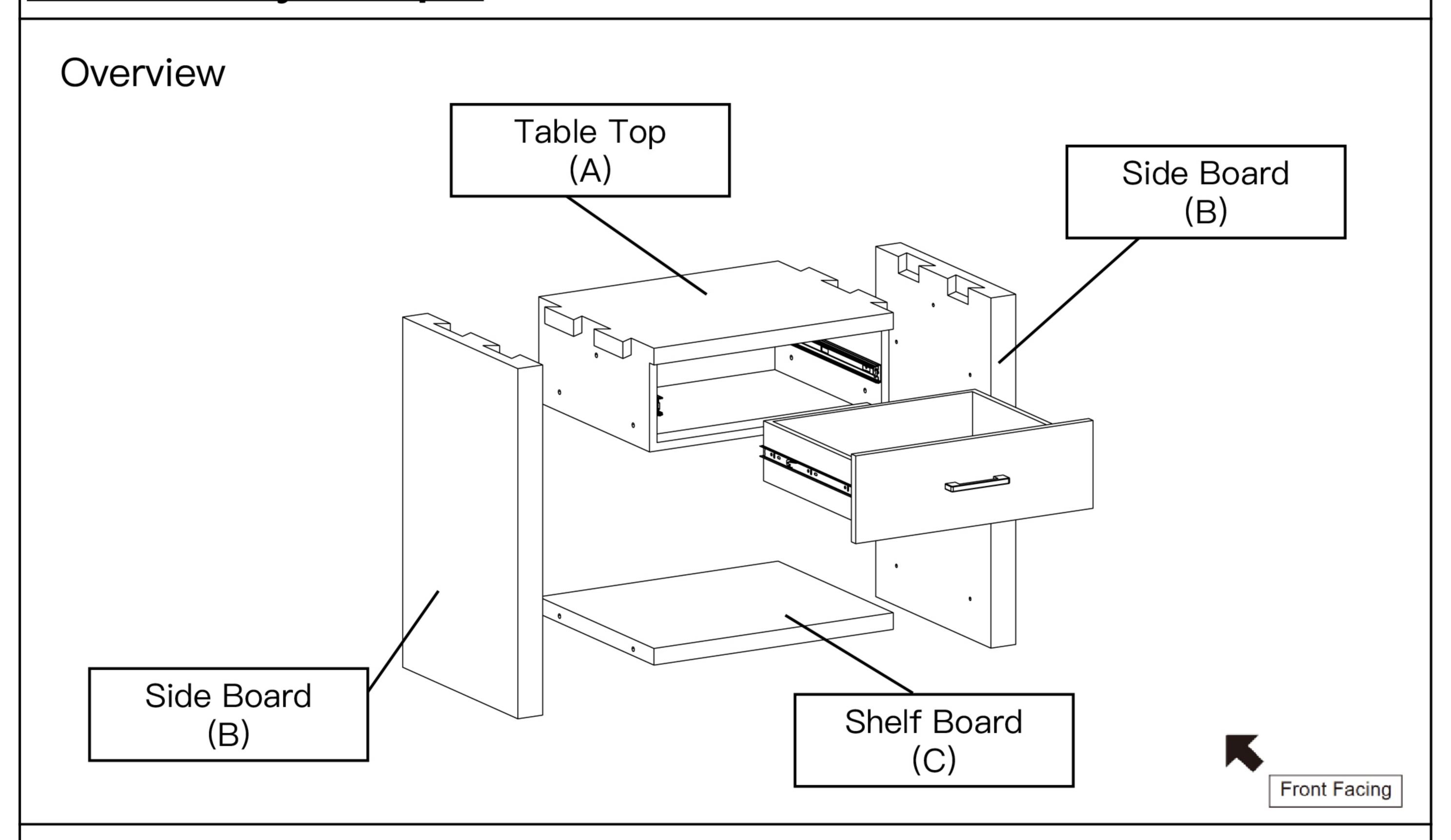
This side table has multiple parts and may require up to some 45 minutes to assemble. To give you an overview of the side table parts, the above picture is to help you put the various parts into perspective. Please read through the instructions below to familiarise yourself with the parts and steps before assembly.
