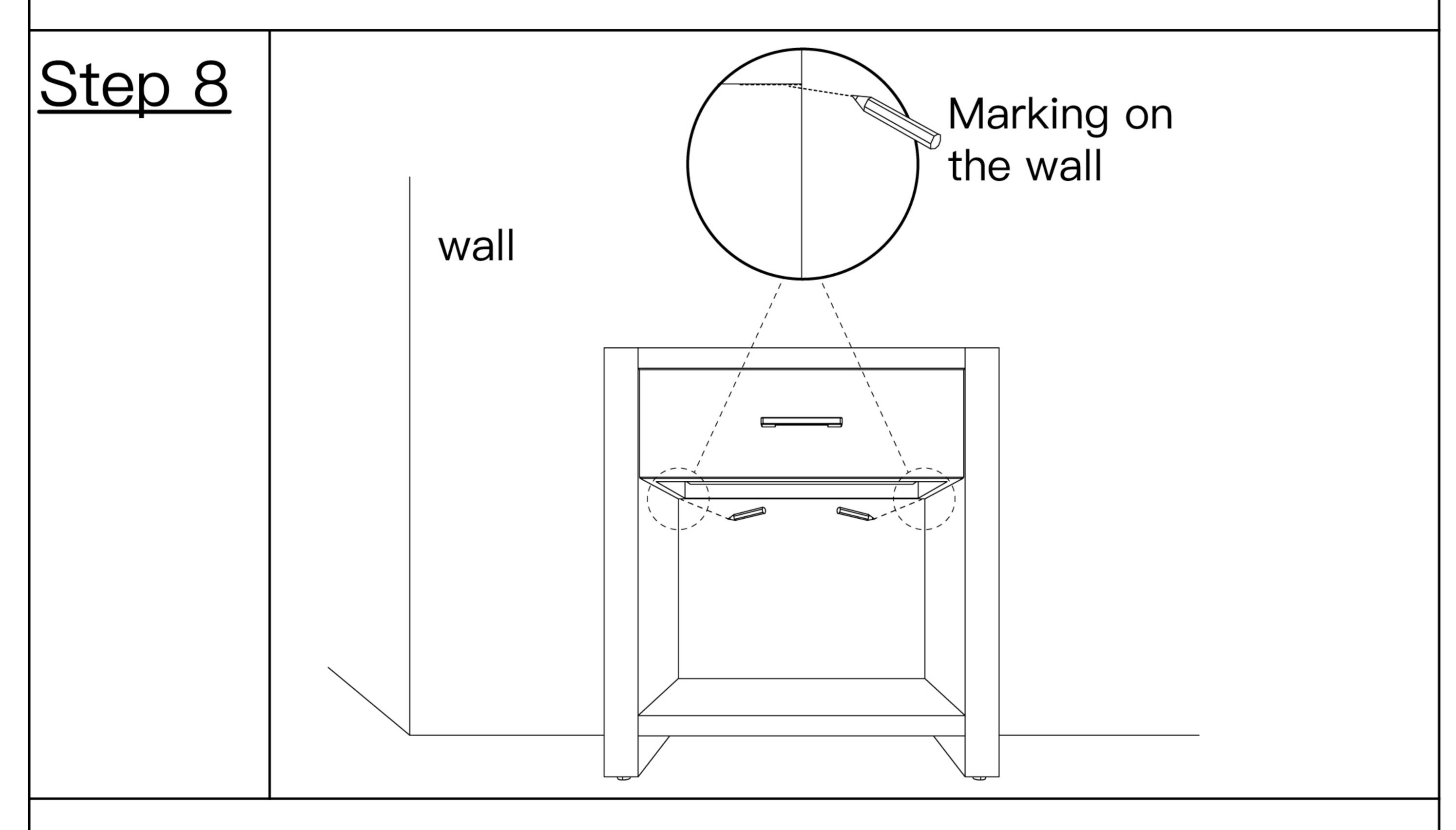
Place the side table against the wall. Mark the positions for the expansion plugs on the wall.
