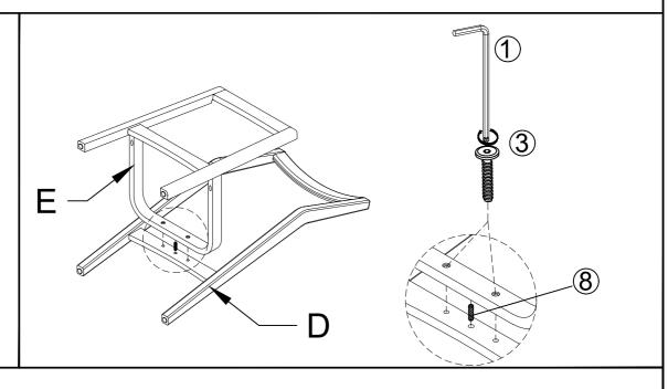
Connect the Connecting Rod (E) into the Rear Leg Frame (D) using the Allen Wrench (1), Bolts (3), Wood dowel (8). Do not fully tighten the Bolts at this time.
