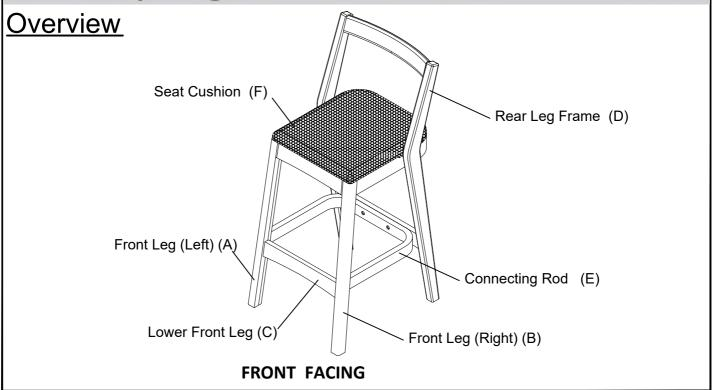
This Bar Stool has multiple parts and may require up to some 30 minutes to assemble. To give you an overview of the chair parts, the above picture is to help you put the various parts into perspective. Please read through the instructions below to familiarise yourself with the parts and steps before assembly.
