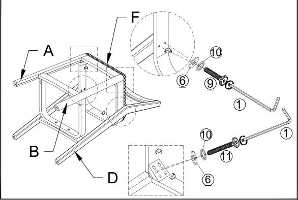
Place the Seat Cushion (F) between the front and back legs, using the Allen Wrench (1), Bolts (11), Spring washer (10), Flat washer (6) to connect the Seat Cushion (F) with the Front Leg (left) (A), Front Leg (right) (B) and the Allen Wrench (1), Bolts (9), Spring washer (10), Flat washer (6) to connect the Seat Cushion (F) with Rear Leg Frame (D). Finally, tighten all the bolts step 4 sequentially.
