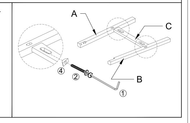
Conecting the Front Leg (left) (A) into the Lower Front Leg (C), Front Leg (right) (B) using the Allen Wrench (1), Bolts (2), Halfmoon washer (4), as pictured above. Tighten the Bolts.
