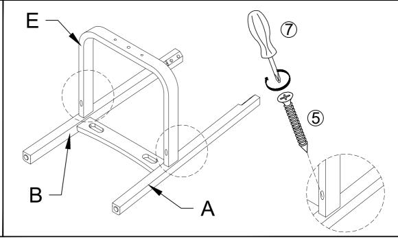
Insert the Connecting Rods (E) into the Front Leg (left) (A), Front Leg (right) (B) using the Screwdriver (7) and Screws (5). Tighten the Screws.
