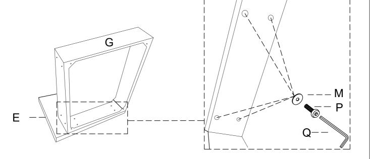
2. Install the seat frame G to the right armrest F with screws
