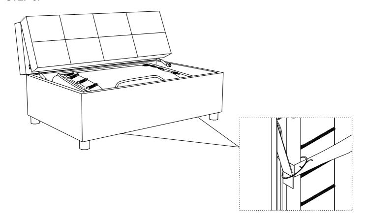
The folding bed assembly has been secured with Tie-wraps for transportation purposes. DO NOT remove the tie-wraps on the front of bars of the assembly until you have finished Step X of the assembly process.
