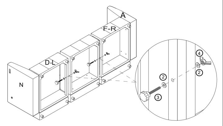
Slip • over • through the connection holes of the two frames, then slip another • over it, and secure it with • hardware.
