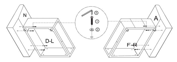
Slip over using to connect N to D-L and A to F-R
