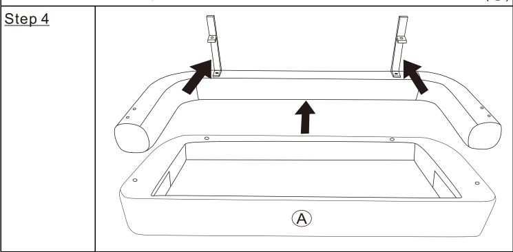
Insert the bottom of the Sofa Frame (A) upwards onto the armrest backrest where the sofa legs have already been installed
