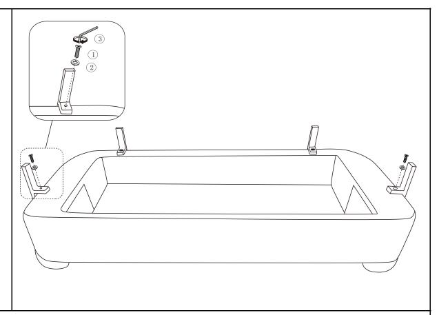
Use Long Screws (1) and Washer (2) to fix the sofa legs respectively. and use a Allen Wrench (3) for fixation
