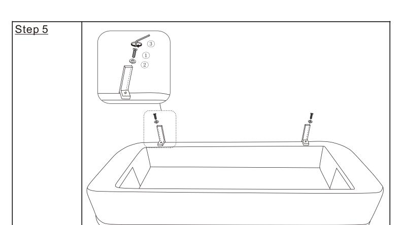
Use Long Screws (1) and Washer (2) to fix the sofa legs respectively. and use a Allen Wrench (3) for fixation
