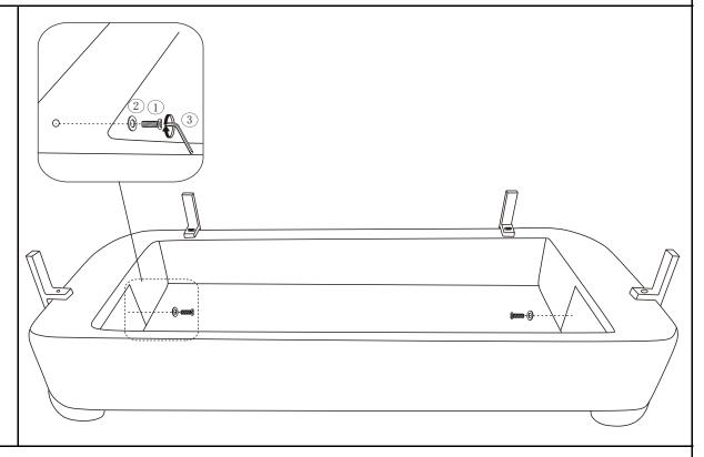
Use Long Screws (1) and Washer (2)Fix the Armest Leg(F) from the inner side of the bottom and use a Allen Wrench (3) for fixation
