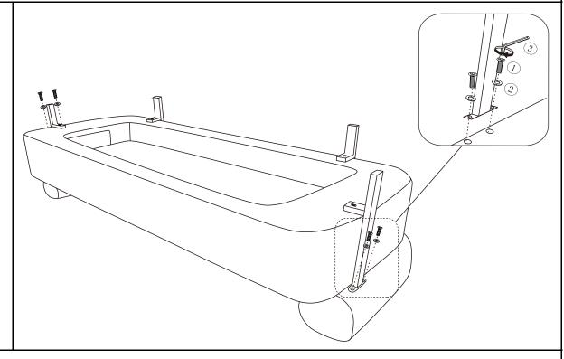
Fix the Armest Leg(F) to the holes on the armrests respectively with Long Screws (1) and Washers (2), and use a Allen Wrench (3) for fixation
