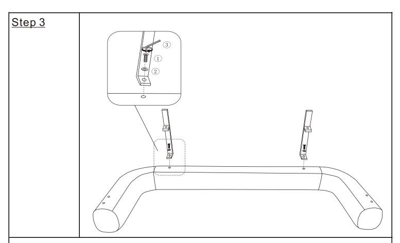
Place the assembled backrest and armrests with the holes facing upwards on the ground.
