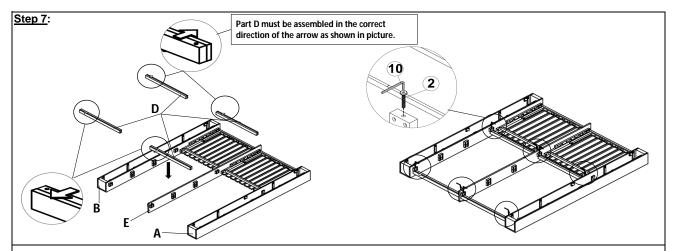
With the help of your adult partner, attach the Second Support Bars (D) to the assembled part in Step 6 by using Screws (②) and Allen Wrench (⑩) as shown above.
