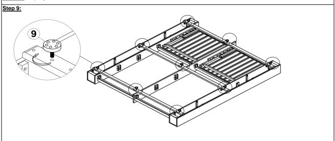
Attach the Levellers (9) to the assembled part in Step 8 by tighten the Levellers counterclockwise as shown above.
