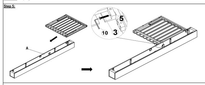
With the help of your adult partner, attach the Left Seat Base Panel (A) to the assembled part in Step 3 by using Bolts (③), Flat Washers (⑤) and Allen Wrench (⑩) as shown above.
