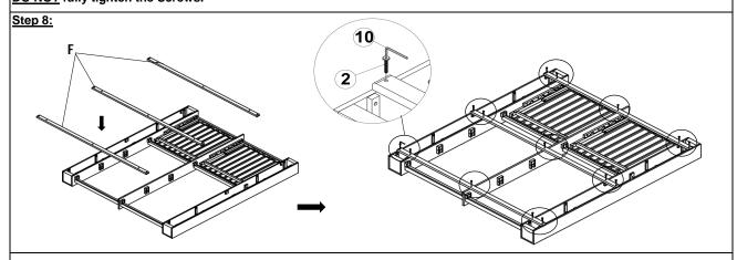
With the help of your adult partner, attach the Feet Base Panels (F) to the assembled part in Step 7 by using Screws (②) and Allen Wrench (⑩) as shown above.
