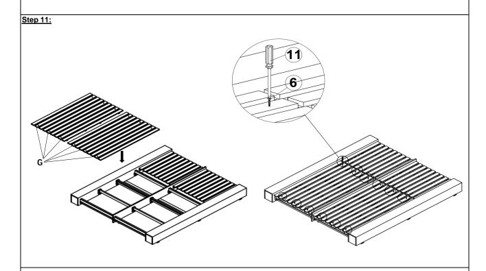
With the help of your adult partner, place the Seat Frames (G) to the assembled part in Step 10 then secure the Seat Frames (G) to the Second Support Bars (D) by using Screws (⑥) with Screwdriver (⑪) as show above picture.
