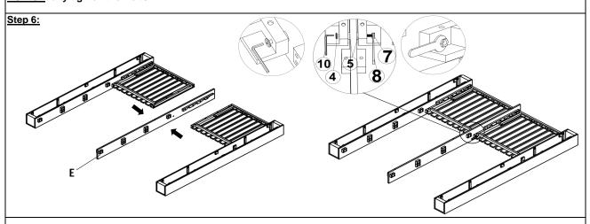
With the help of your adult partner, attach the assembled parts in Step 4 & 5 and Middle Bar (E) together and then secure by using Bolt (④), Flat Washers (⑤), Lock Nut (⑦), Wrench (⑧) and Allen Wrench (⑩) as shown above.
