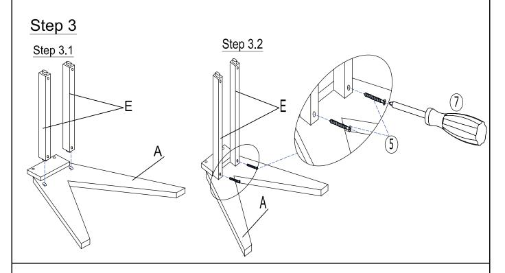
Place the Left Leg Panel (A) lie as shown in the picture above onto a clean, soft surface to avoid any scratches or damage to the product. With assistance from your adult partner(s): Attach the Support Bar (E) to the Left Leg Panel (A), using Screws (5) and the Screw Driver(7) (Not provided) as shown above.
