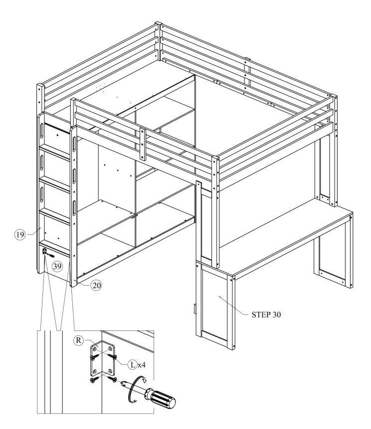
Install Patt L (R) into 2 positions with pre-drilled guide holes as shown.
