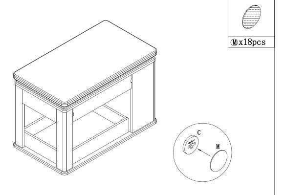
After installing the product, label the corresponding number M according to the color of the components At the perforation location
