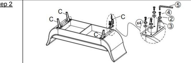
Attach the Leg (C) to Seat Frame(A) and Side frame (B) by using Bolts (4),Spring Washer(2),Flat Washers(3) with Allen Wrench(5).
