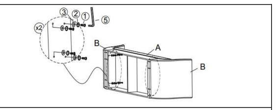
Attach Seat Frame(A) to Side frame (B) by using Bolts(1),Spring Washer(2), Flat Washers(3) with Allen Wrench(5).
