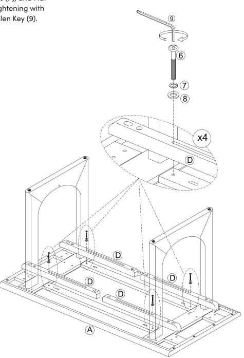
Next, tighten the outer round holes of the Extension Leaf Supports (D) to the corresponding holes on the Tabletop (A) using the Hex Button Head Bolts (5), Spring Washers (7), and Flat Washers (8). Tighten them with the Allen Key (9).
