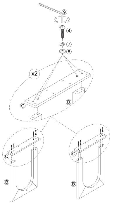
Next, attach the leg assemblies (B) completed in Step 1 to the Tabletop (A) using the Hex Button Head Bolts (4), Spring Washers (7), and Flat Washers (8). Tighten them with the provided Allen Key (9).
