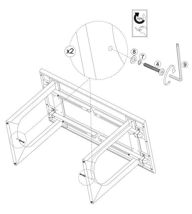
Now, place the Round Bottom Stretcher (E) onto the two bolts that were loosely attached in Step 7, then tighten them.
