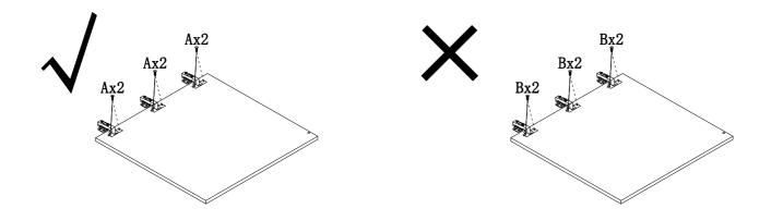
NOTE-2: Please note that this product contains multiple screws. When connecting the door panel and the side panel, be sure to use the shortest screw, type A. Using the wrong screw may cause damage to the plate parts.
