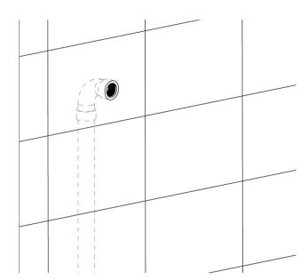
4.Install the connecting leg, wrapping the threads with plumber's tape for a secure seal.
