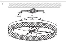
Rotate the Iamp body to align the screws on the mounting plate with the holes on the leftmost hub.
