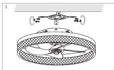
Tighten the four screws on the mounting plate to ensure the fixture ie securely instlled.
