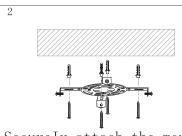
Securely attach the mounting plate to the ceiling.
