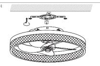
Rotate the Iamp body to align the screws on the mounting plate with the holes on the leftmost hub.
