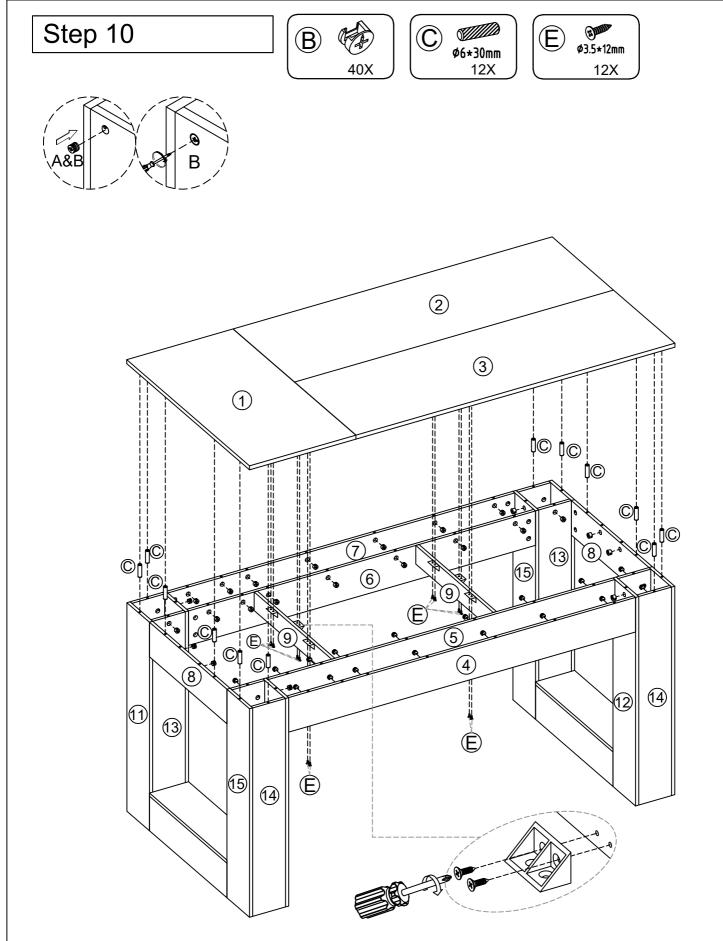
Ais already locked in the panels 123 in advance, simply lower the panel to place into the corresponding holes, as shown: hole corresponding to the lock plate B
