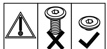
The screws are completely tightened.
