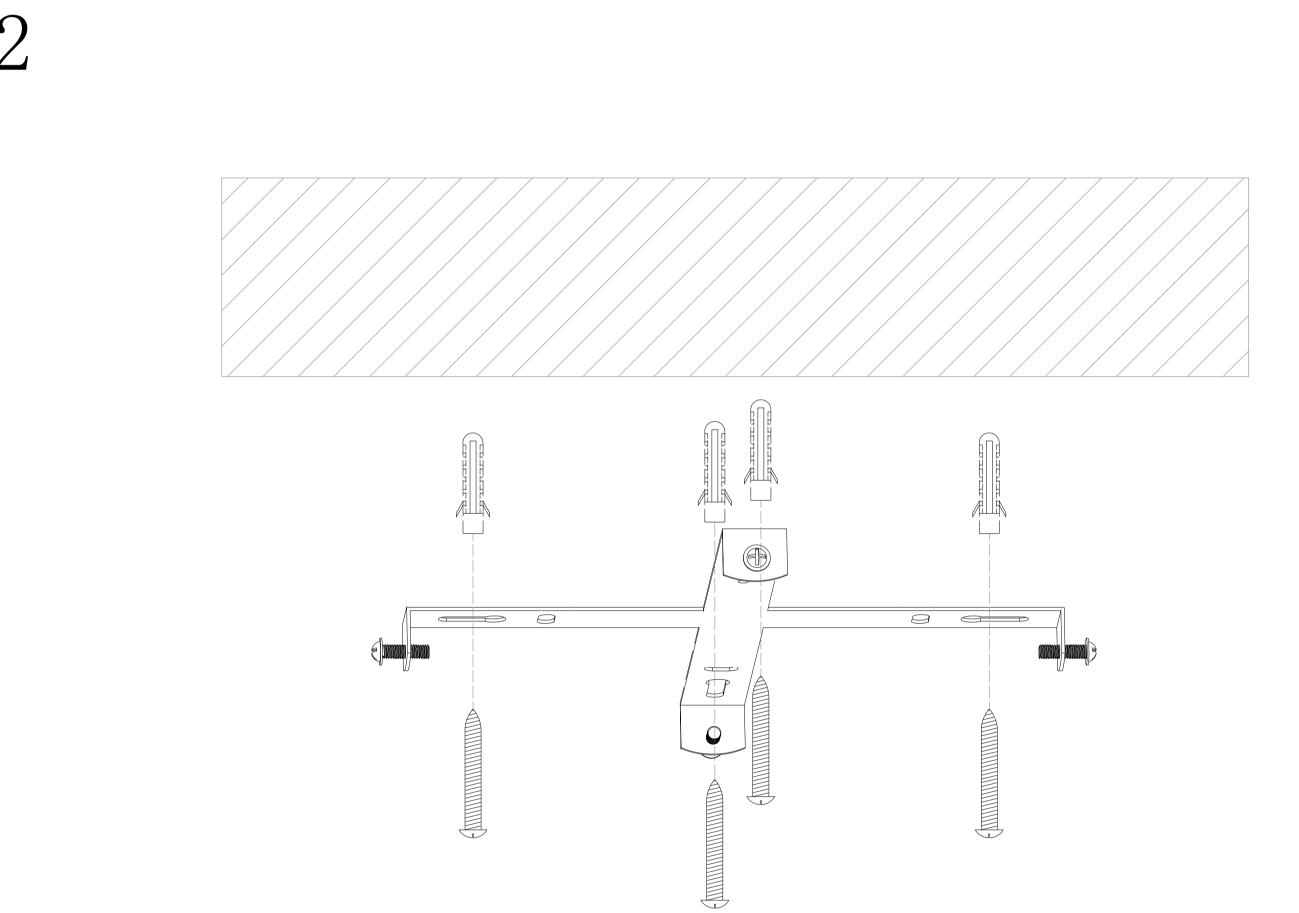
Securely attach the mounting plate to the ceiling.
