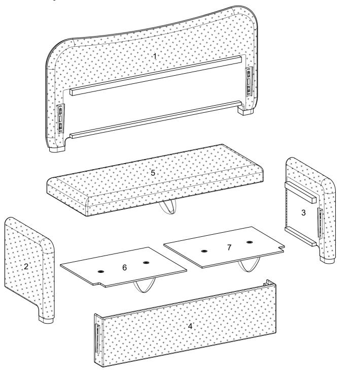
Connect the Left Side Frame (2) to the Back Cushion (1) by sliding it into place with the attached hardware.
