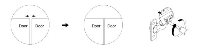
If the gap is too tight between the two doors, loosen the screw at the front of the hinge as shown to make the adjustment and then re-tighten the screw.
