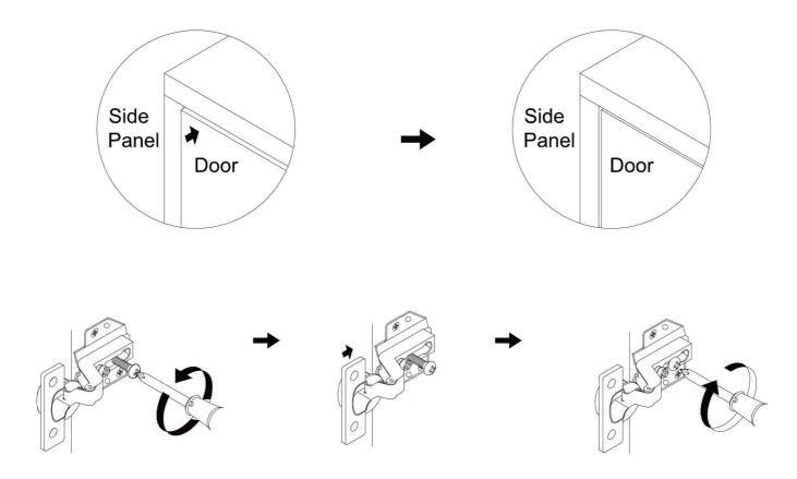
If the top of the door is not level with the side panel, loosen the screw at the back of the hinge as shown, then move the hinge in or out until the desired gap is achieved, and then re-tighten the back screw.
