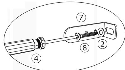
Attach Metal Brackets (7) to Wall Plugs (9) using Wall Plug Screws (8) and Washer (2) with Screwdriver (4).
