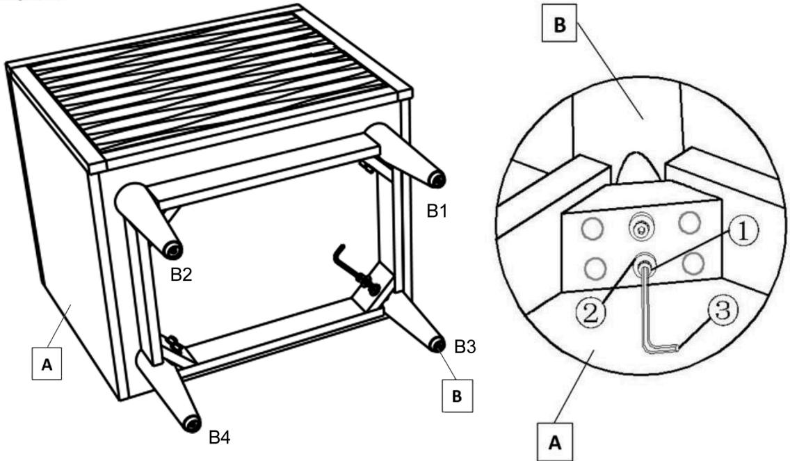
As shown in "Step 2" picture attach the Leg (B1,B2,B3 & B4) into the Top (A) by using Allen Bolt (①), Washer (②) and Allen Wrench (③).
