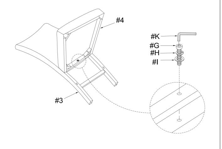
Do not tighten screws until completely asembled.
