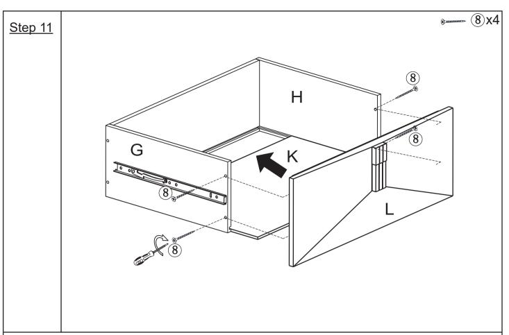
Insert drawer botton panel(K) into the groove of drawer left panel(G) and drawer right panel(H). Attach drawer panel(L) to drawer left panel(G) with screw ( $\otimes$ ) using screwdriver. Repeat the previous steps to drawer right panel(H).
