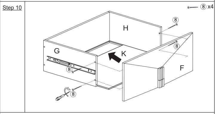
Insert drawer botton panel(K) into the groove of drawer left panel(G) and drawer right panel(H). Attach drawer panel(F) to drawer left panel(G) with screw (®) using screwdriver. Repeat the previous steps to drawer right panel(H).
