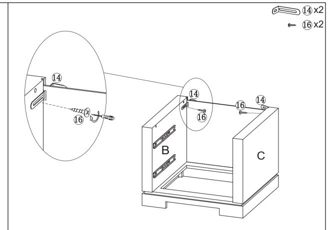
Attach the long side of anti-tipping sheet iron ( 14 ) into left side panel(B) with screw(16) using screwdriver.
