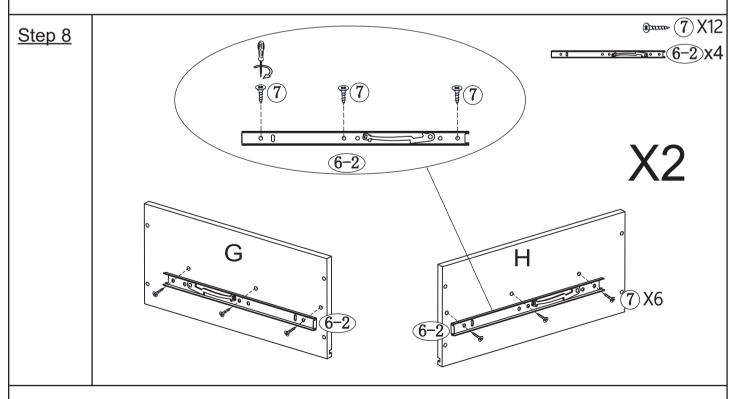
Attach the slide rail ( 6-2) to drawer left panel(G) with screw(7). Repeat the previous steps to drawer right panel(H).
