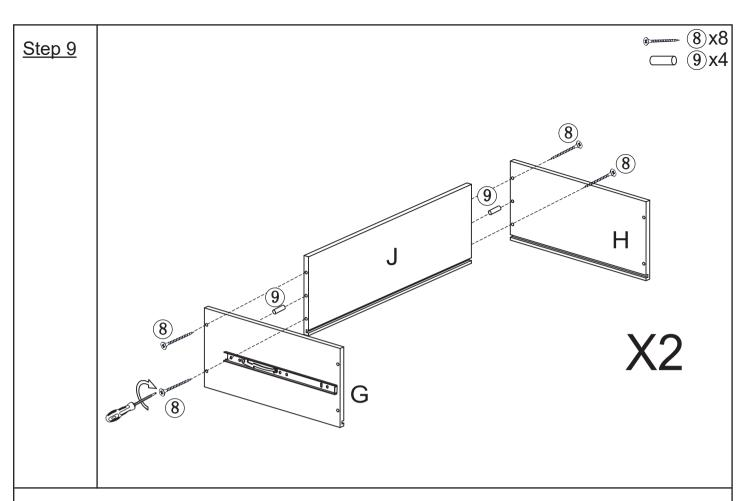
Attach drawer left panel(G) to drawer back panel (J) with screw (®) and dowel(9) using screwdriver. Repeat the previous steps to drawer right panel(H).
