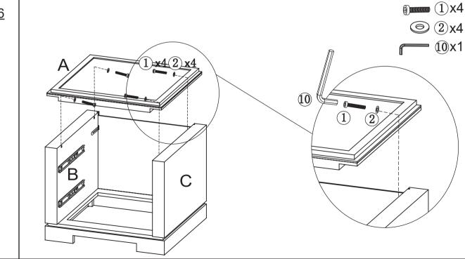
Attach the top panel (A) to the left side panel(B) with bolt (1) and flat washer(2) using allen wrench(10).
