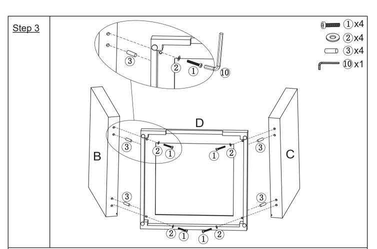
Attach the bottom panel (D) to the left side panel(B) with bolt(1),flat washer(2) and dowel(3) using allen wrench(1). Repeat the previous steps to right side panel(C) .
