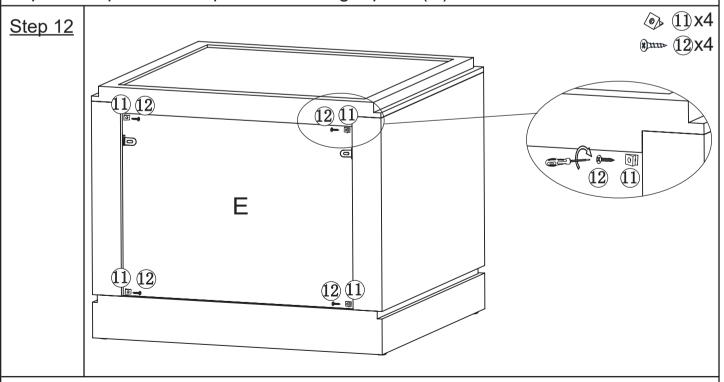
Attach plastic button((1)) into the back panel(E) with screw((1)) using screwdriver.
