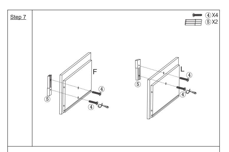
Attach knob (5) to drawer panel (F) with bolt (4) using screwdriver. Repeat the previous steps to drawer panel (L).
