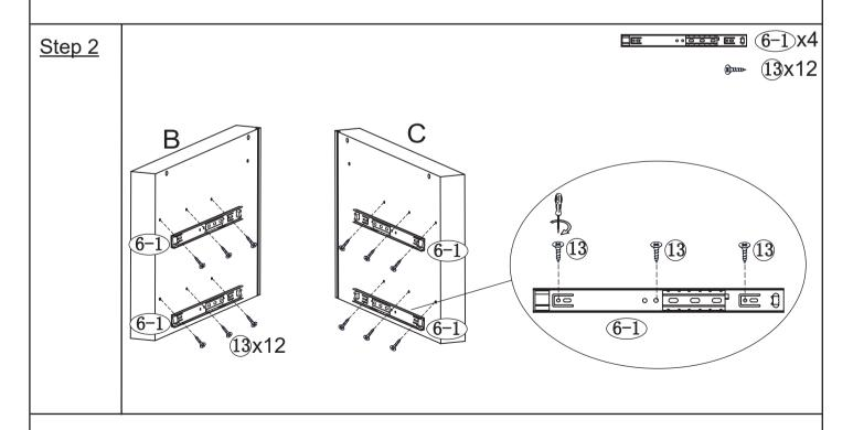
Attach the slide rail (6-1) to left side panel(B) with screw(13). Repeat the previous steps to right side panel(C).
