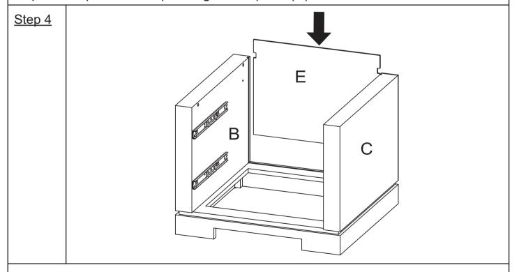
Insert back panel(E) into the groove of left side panel(B) and right side panel(C).
