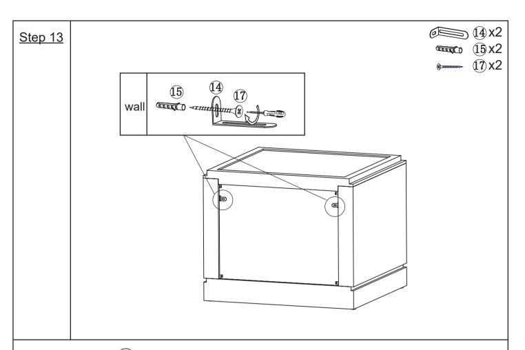
Screw the nut (  $\bigcirc$  ) into the wall. Install the short side of anti-tipping sheet iron(  $\bigcirc$  ) on the wall with screw(  $\bigcirc$  ) using Screwdriver.
