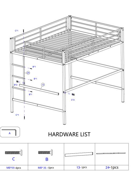
Step 8:Place the materials on the ground according to the figure.
