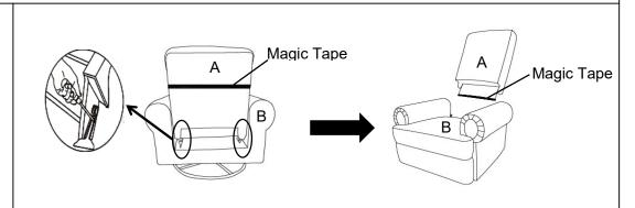
Disassembly Note:Open the flap on the Chair Backrest(A),use a screwdriver(Don't use fingers) pressing outward on the metal ear on the preattached Metal Bracket on one side of the Chair Base(B),with assistance of you adult partner to keep the Chair Base(B) in place, pull out the Chair Backrest(A) upward at the same time,repeat the same step for another side. Then the Chair Backrest(A) can be taken out.
