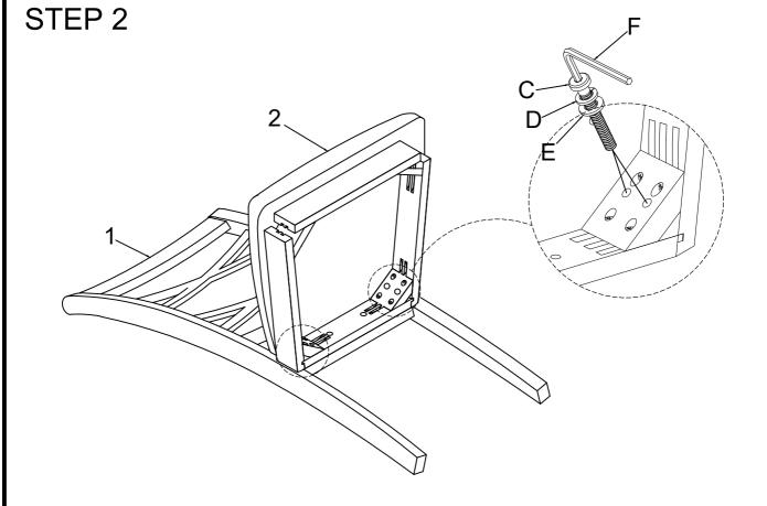
Do not tighten screws until completely assembled.
