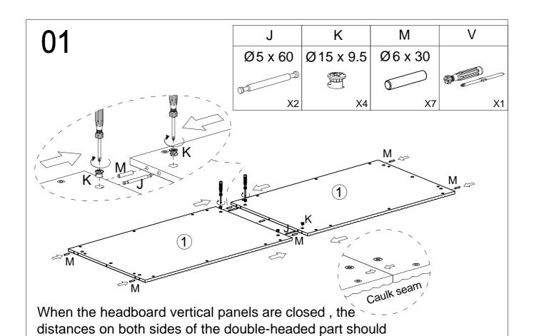
be symmetrical. Place the three-in-one plate and lock the
