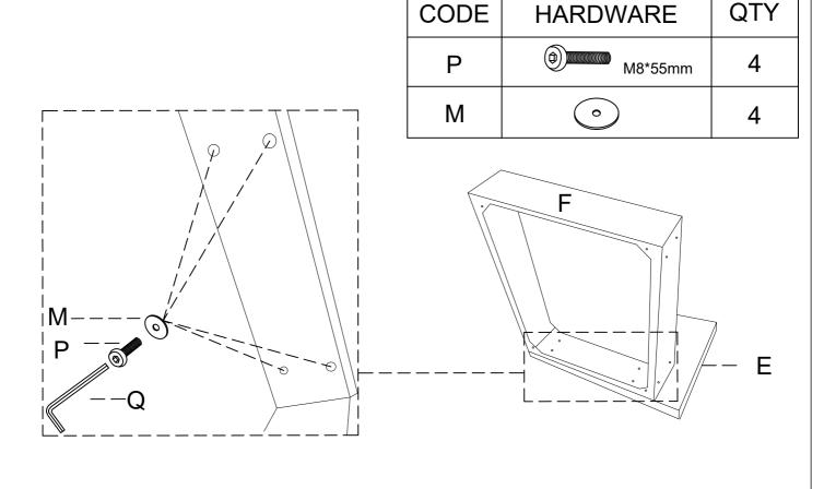
3. Connect the seat frame F with screws P, washers M and
