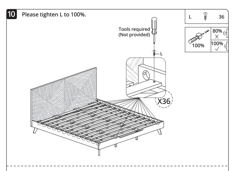
If it feels uneven on the floor, first tighten all the screws, then adjust the leveling feet of Slat Supporting legs (9) for balance.
