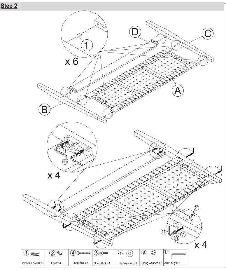
Align the mounting position of Headboard (A) ,Cross Panel (D) and two Headboard Legs (B) & (C) with wooden dowel (1).
