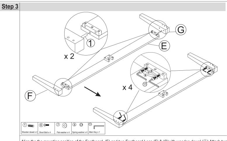
Align the the mounting position of the Footboard (E) and two Footboard Legs (F) & (G)with wooden dowel (1). Attach two Footboard Legs (F) & (G) to Footboard (E) by using a short Bolt (6), Spring Washers (8) and Flat Washers (7) with Allen Wrench(1).
