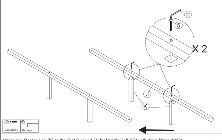
Attach the Center Leg (K) to the Slat Support (J) by Middle Bolt ( ${\mathfrak D}$ ) with Allen Wrench( ${\mathfrak Q}$ ) .
