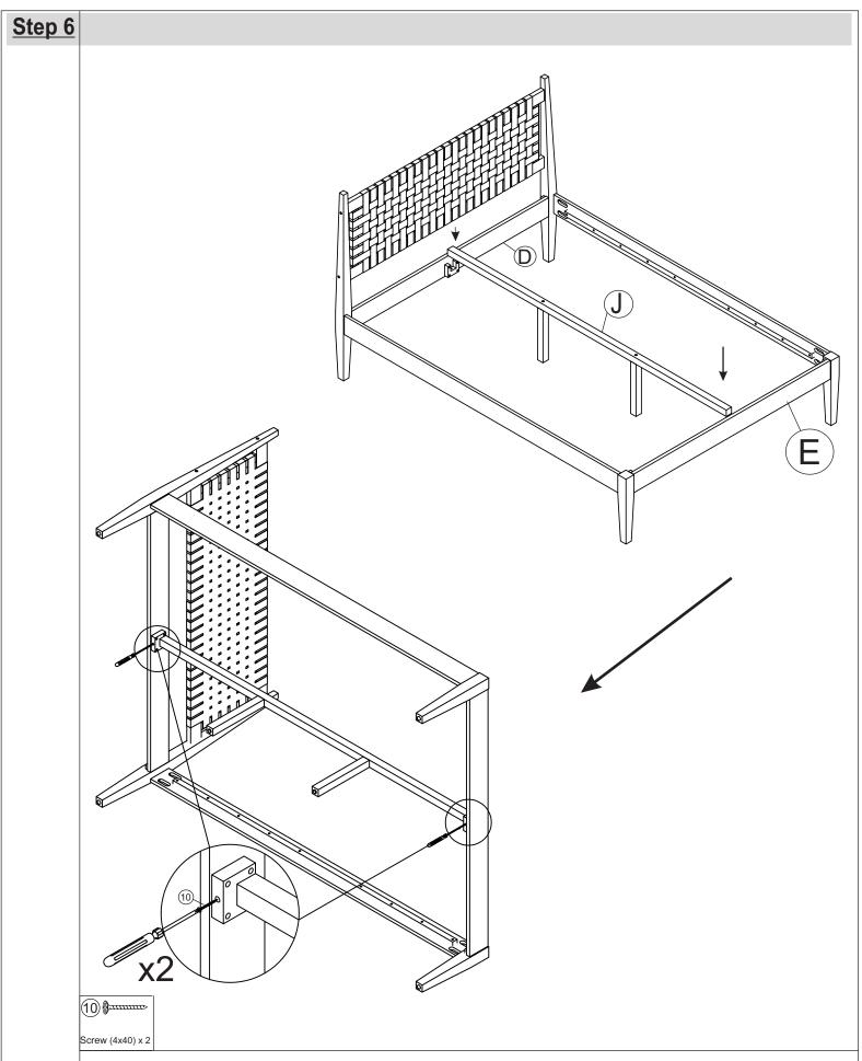
Attach the Slat support (J) to the Cross Panel (D) and Footboard (E) by using Screw (1) and Screwdriver (Not Provided).
