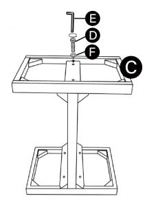
Attach table base C to the end of leg B with screws and flat washers as shown.
