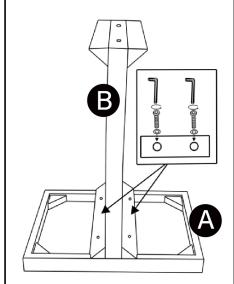
Flip the table top A upside down. Attach leg B to the bottom of table top A with screws and flat washers as shown.
