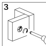
3: On the back of the Cam Lock will be a "C" shape. Insert the Cam Lock so the opening of the "C" fits over the Cam Bolt. Tighten with the screwdriver.
