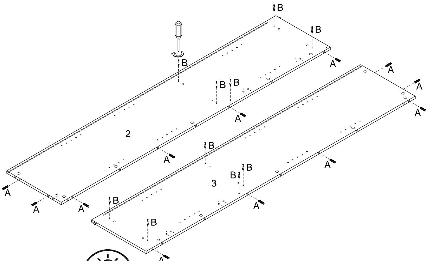
1: The provided glue is to secure wood dowels in place. When first inserting dowels, locate the appropriate hole for the dowel, place a small amount of glue in the hole and insert the dowel. Wipe away excess glue immediately.
