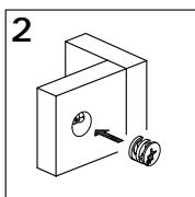
2: Fit the proper holes on the edge of the other part over the Cam Bolts. You should be able to see the cam bolts through the larger hole on the side.
