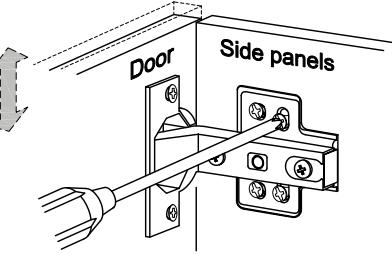
Adjust vertical height via the screws in the mounting plate.
