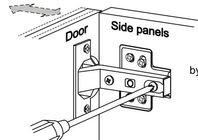
Adjust depth position by loosening the hinge arm mounting screw.
