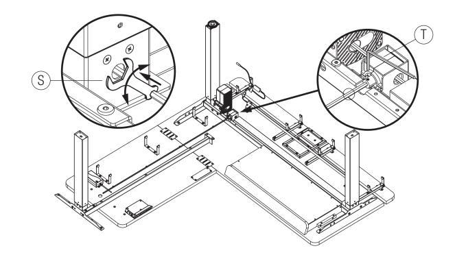
Fine-tune with the aid of a Hex Wrench (S) if necessary to align the Hexagonal Shaft to the hole. Do not make large adjustments. If the correction is excessive, set the metal foot to the lowest possible level and retune.
