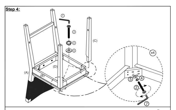
Next, attach the Front Legs (C) & (D) to the Seat frame (B) using the Bolt (2), Lock Washer (4) & Flat Washer (5) with Allen Wrench (7)
