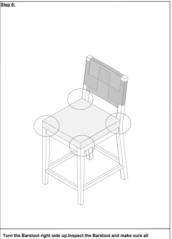
Turn the Barstool right side up.Inspect the Barstool and make sure all parts are adequately connected. joints.In a sequential manner, tighten all Bolts and Screws at all joints.
