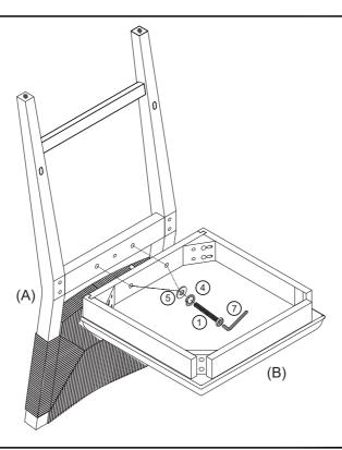
With assistance from your adult partner, connect Seat frame (B) to Back frame (A) using the bolt (1), Lock washer (4), Flat washer (5), with Allen Wrench (7)
