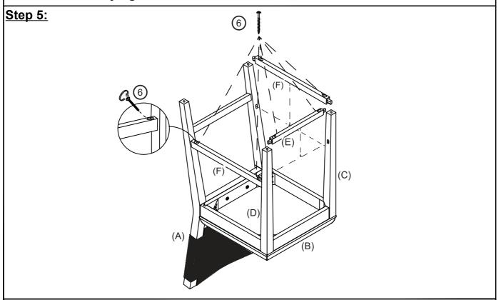
Now, connect Front Footrest (E) and Side Stretchers (F) using screw 6. If you are having trouble getting the screws to catch, it is recommended to carefully use an electric screwdriver or drill with necessary bit for this step.
