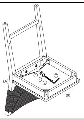
Match the sticker on the bottom of the Back frame (A) with the sticker on the corner block of the Seat frame (B).
