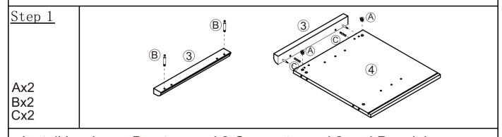
Install hardware B onto panel 3. Connect panel 3 and Panel 4 with hardware A and C.
