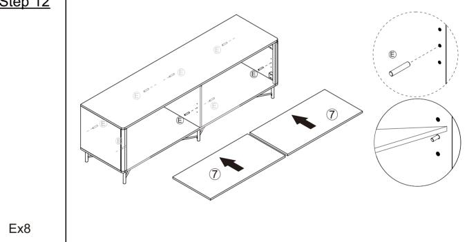
Hardware E inserted in the hole.Put laminate 7 in.
