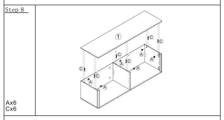
Connect the top plate 1 to the panels 2,4,6 with hardware A and dowels C.
