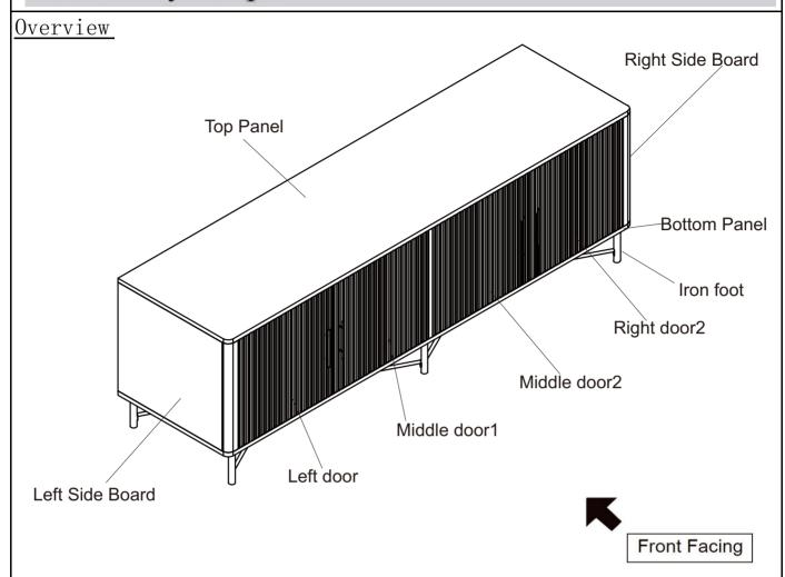
This Cabinet has multiple parts and may require up to 50 minutes to assemble. To give you an overview of the cabinet parts, the above picture is to help you put the various parts into perspective. Please read through the instructions below to familiarise yourself with the parts and steps before assembly.
