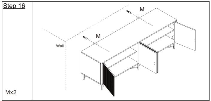
Cabinet must permanently fixed to the wall with included anti-tipping device to prevent the cabinet from tipping over. Mark the drill position on the wall with a pencil. Drill holes on the marked position using a bit. Gently inert the wall anchor (M) into the drilled hole with the help of a hammer Fixed the cabinet to the wall with provided screws (M)
