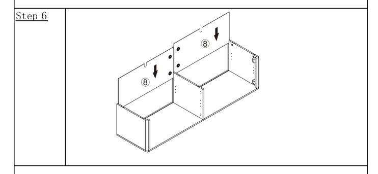
Flip the product from step 5 to the right as shown in the figure. Insert the backing plate 8 through the slot
