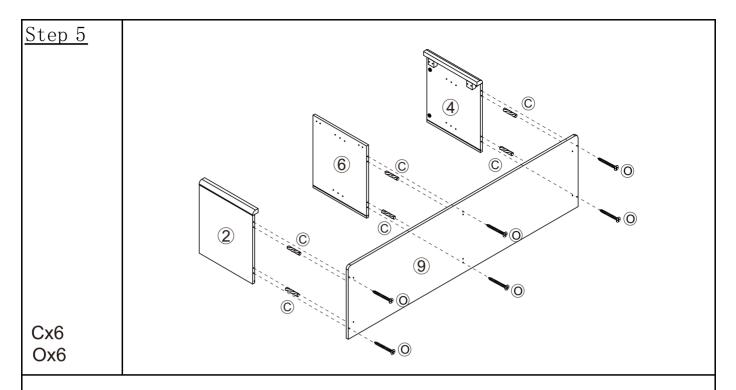
Connect Panel 2, Panel 4 and panel 6 to Panel 9 with hardware C and hardware O.
