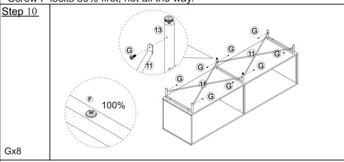
Connect iron 12 and iron 13 to iron 11 with hardware G. Tighten screws G all the way and finally lock screws F.
