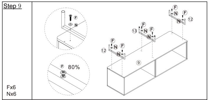
Flip the cabinet from step 8 so that the bottom is facing up as shown. Attach the assembled iron feet to the base plate 9 with hardware F/N. Screw F locks 80% first, not all the way.
