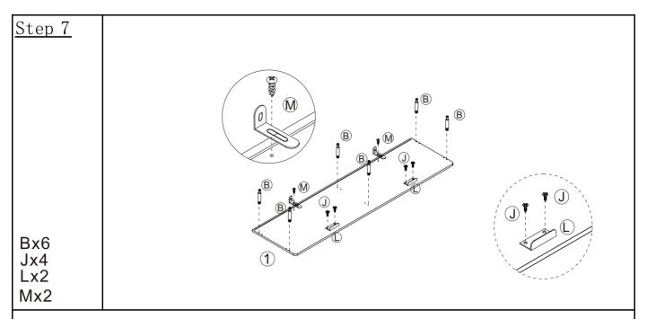
Lock hardware B to plate 1. Fix the anti-toppling M to the panel 1. Secure the hardware L to the top of the plate 1 with screws J.
