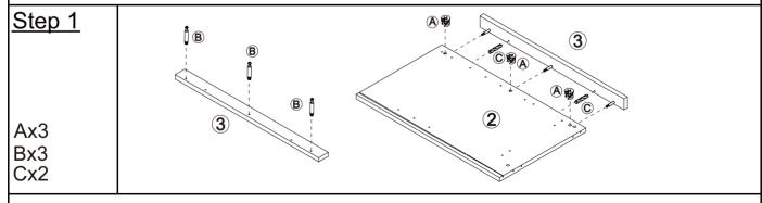
Install hardware B onto panel 3. Connect panel 3 and Panel 2 with hardware A and C.
