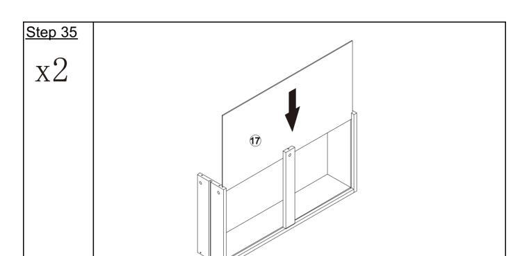
Insert the drawer base 17 into the slot. Repeat this step 2 times.
