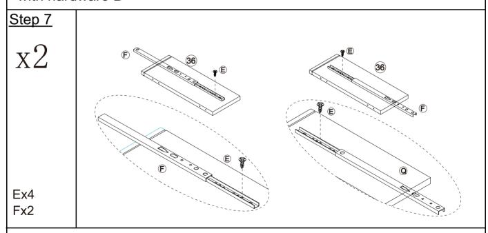
Secure the slide F to the plate 36 with screws E.
