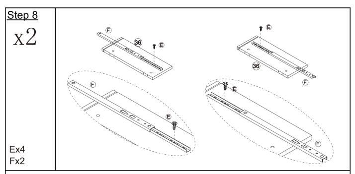
This is the other side of Panel 36. Secure the slide F to the plate 36 with screws E.
