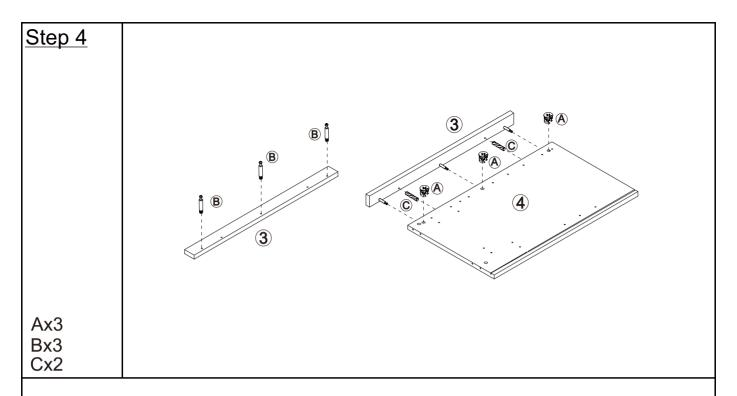
Install hardware B onto panel 3. Connect panel 3 and Panel 4 with hardware A and C.
