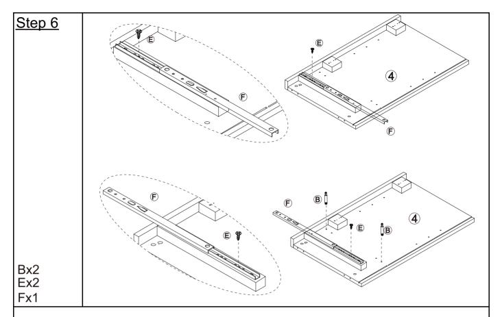
Secure the slide F to the plate 11 with screws E.Attach to plate 4 with hardware B
