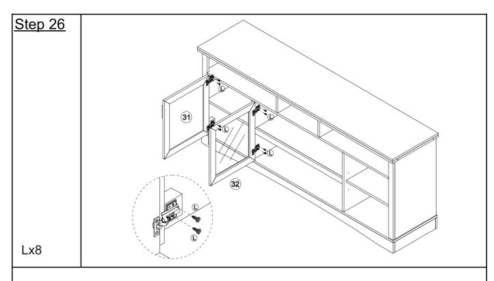
Attach the fitted door to the frame.
