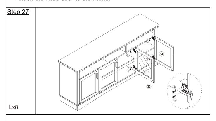
Attach the fitted door to the frame.
