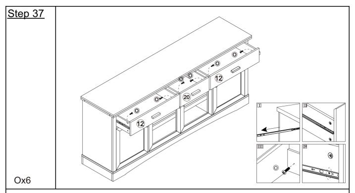
Pull the rails out and put the drawers in, taking care to align the holes. Lock with screw O. Attention: Be careful when pulling the slide, it's best to wear gloves.
