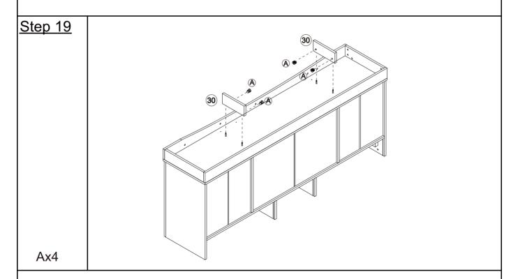
Attach the support plate 30 to the base plate 24 with hardware A.
