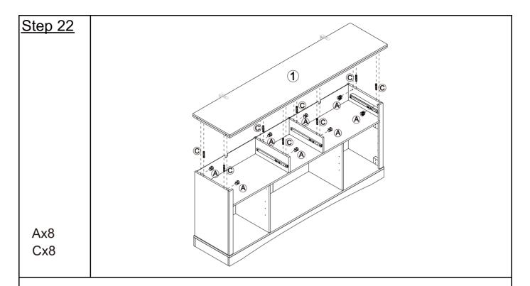
Secure the top plate to the frame with hardware A and dowel C.
