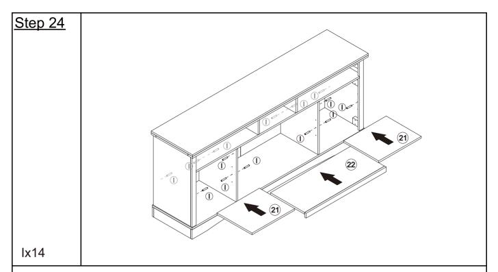
Place laminate pegs I into the holes. Boards 21 and 22 should be placed along the diagonal of the cabinet.
