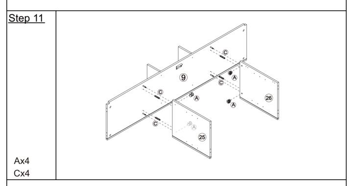
Secure plate 25 and plate 26 to plate 9 with hardware A and dowels C.
