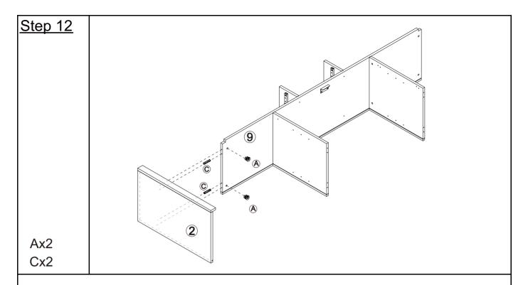
Secure plate 2 to plate 9 with hardware A and dowels C.
