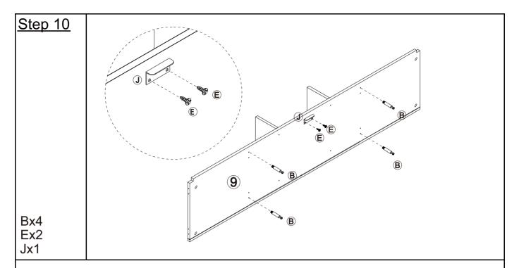
Fasten Hardware B to Plate 9 and Fasten Hardware J to Plate 9 with Screw E.
