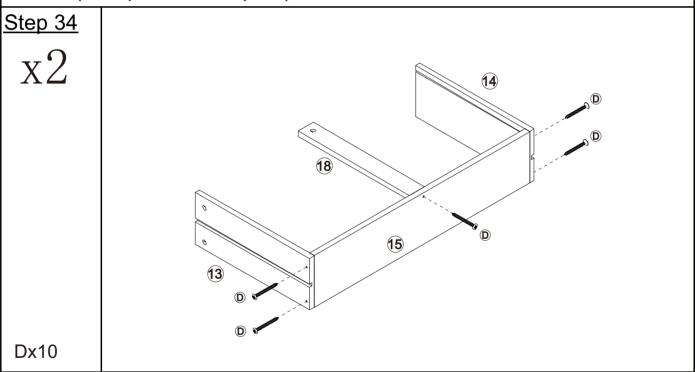
Attach plate 13 and plate 15 and plate 18 to plate 14 with screws D. Repeat this step 2 times.
