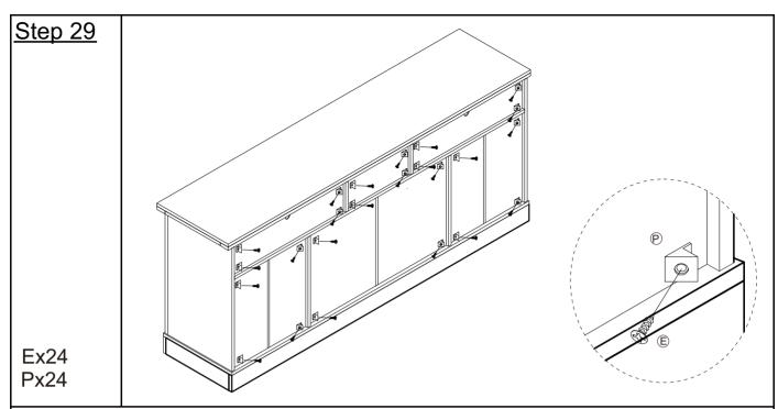
Insert the back panel buckle P into the gap and secure it with screw E.
