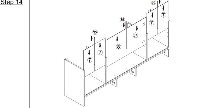
Flip the product from step 13 to the left as shown. Insert the backplate 7 and backplate 8/37 into the slots and the backplate strip 35 into the center of the two backplates.
