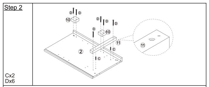
Attach plate 11 to plate 2 with screws D and dowels C, paying attention to the orientation. Attach the plate 10 to the plate 2 with screws D
