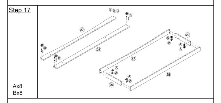
Hardware B mounts to plate member 27 and plate member 28. Connect plate member 27 and plate member 28 to plate member 29 with hardware A.
