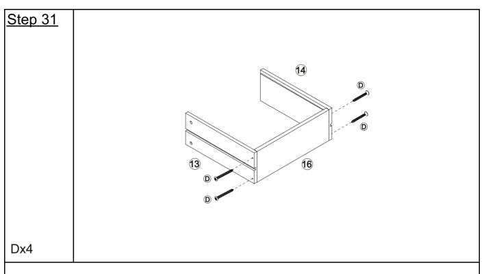
Attach plate 13 and plate 16 to plate 14 with screws D.
