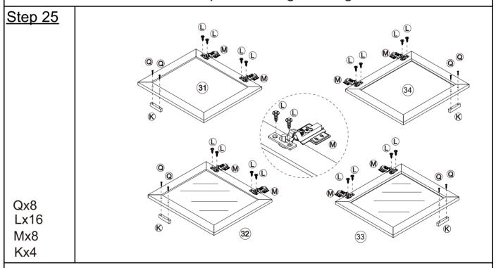
Attach the pull handle K to the door with screw Q and the hinge M to the door with screw L.
