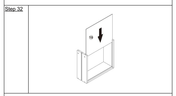
Insert the drawer base 19 into the slot.
