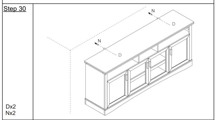
Cabinet must permanently fixed to the wall with included anti-tipping device to prevent the cabinet from tipping over. Mark the drill position on the wall with a pencil.Drill holes on the marked position using a bit.Gently inert the wall anchor (N) into the drilled hole with the help of a hammer Fixed the cabinet to the wall with provided screws (D)
