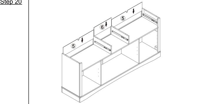
Flip the product from step 19 as shown. Insert the backplate 5 and backplate 6 into the slots.
