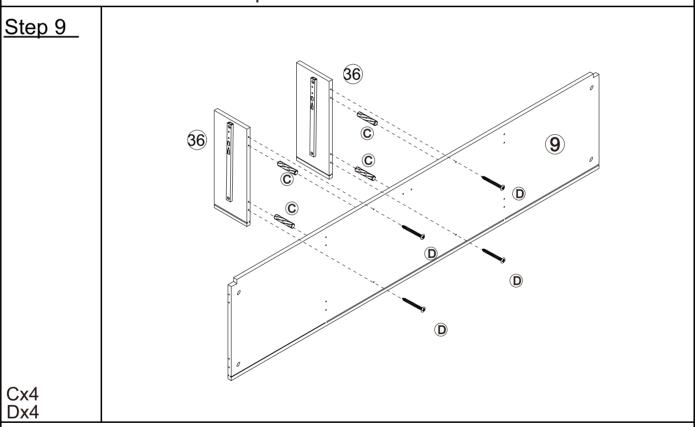
Attach plate 36 to plate 9 with screws D and dowels C
