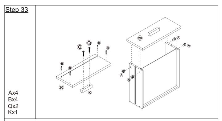
Attach pulls K to the drawer panel 20 with screws Q and hardware B to the drawer panel 20. Attach the drawer panel 20 to the assembled frame (Completed in step 32) with hardware A.
