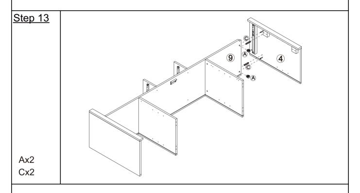
Secure plate 4 to plate 9 with hardware A and dowels C.
