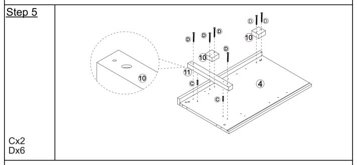
Attach plate 11 to plate 4 with screws D and dowels C, paying attention to the orientation. Attach the plate 10 to the plate 4 with screws D.
