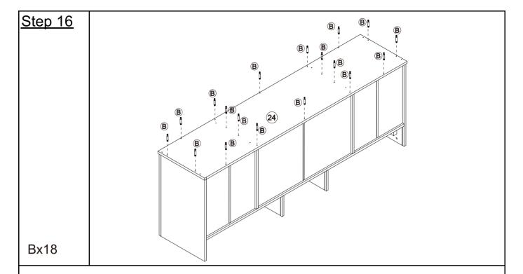
Attach hardware B to base plate 24.
