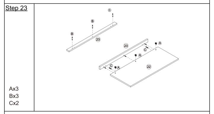
Attach hardware B to plate 23.Use hardware A and dowels C to join plate member 23 to plate member 22.
