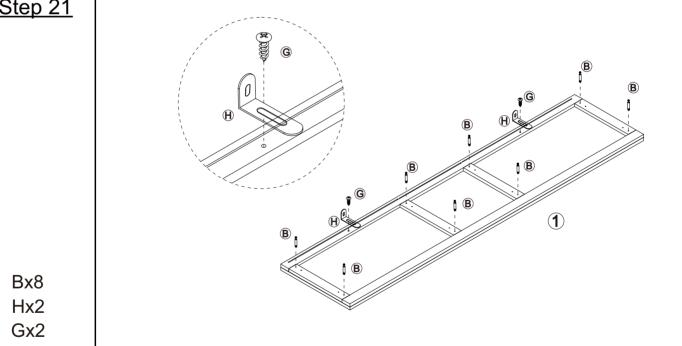
Installation of anti-tipping ,Attach the hardware H to the top of the top plate 1 with screws G. Install the hardware B on top of the top plate 1.
