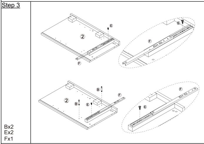
Secure the slide F to the plate 11 with screws E.Attach to plate 2 with hardware B
