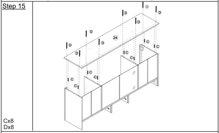
Attach base plate 24 to frame with screws D and dowels C.
