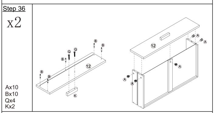
Attach pulls K to the drawer panel 12 with screws Q and hardware B to the drawer panel 12. Attach the drawer panel 12 to the assembled frame (completed in step 35) with hardware A. Repeat this step 2 times.
