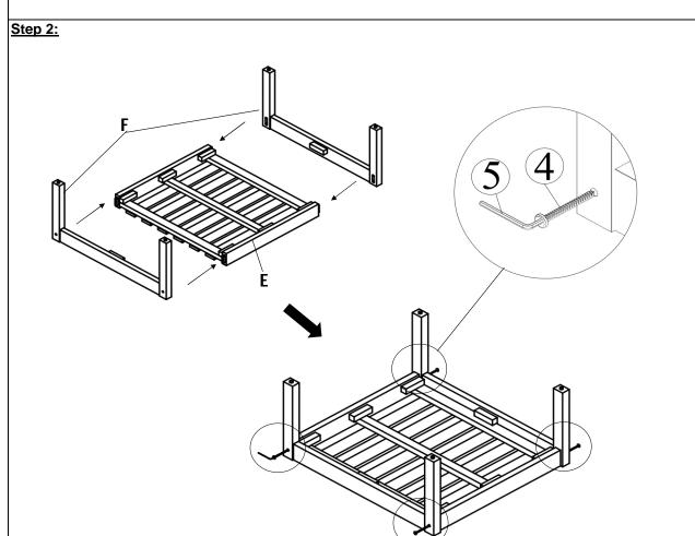
Attach the Leg Panel (F) to the Seat Panel (E) then secure by using Screws (4) with Allen Wrench (5) as shown in the picture above.
