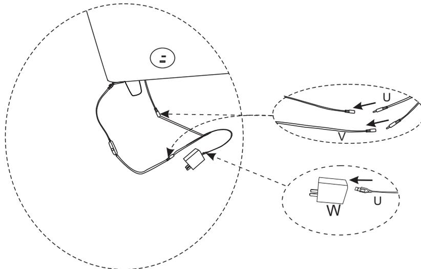
Under the sofa, install the light belt in the front circle, and connect the power switch plug
