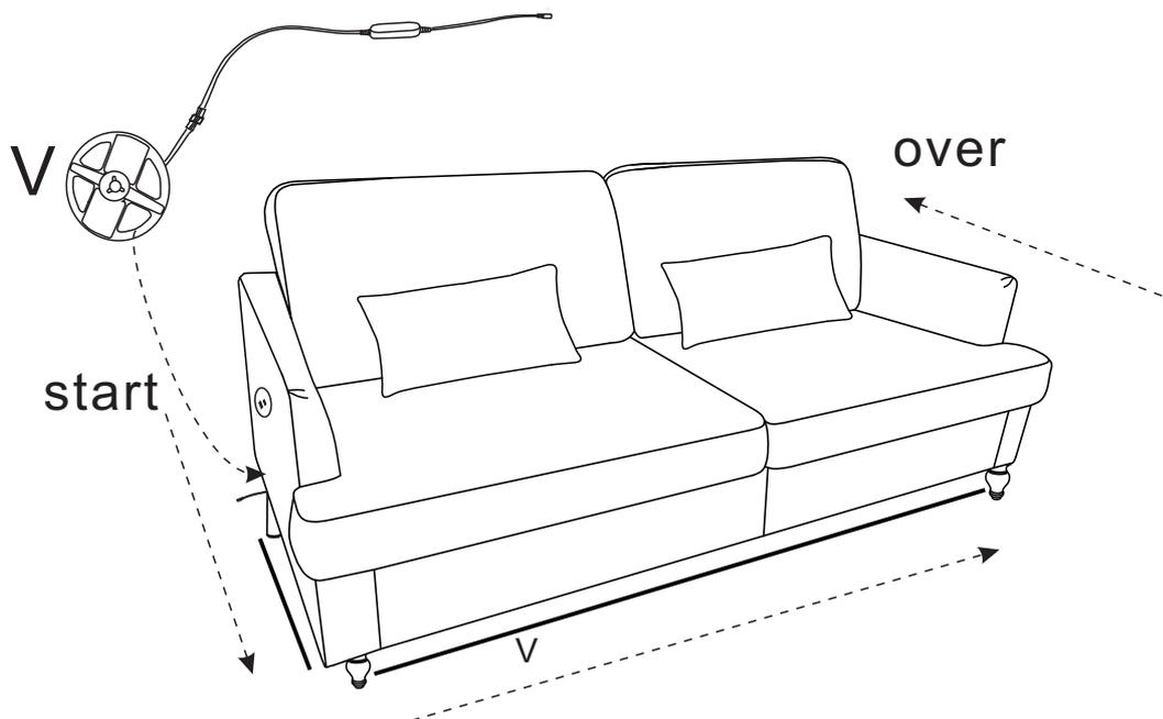
Under the sofa bottom, install the light belt in the front circle and connect the power switch plug
