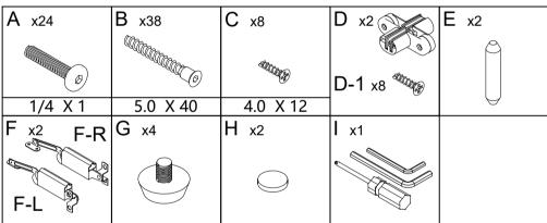
When the process of product assembly, please do not lock the screws at one time, but wait until all the screws are assembled to the position, and then straighten and flatten the product, and then tighten the screws of the same height in turn, so as to avoid unsmooth assembly and product tilt.
