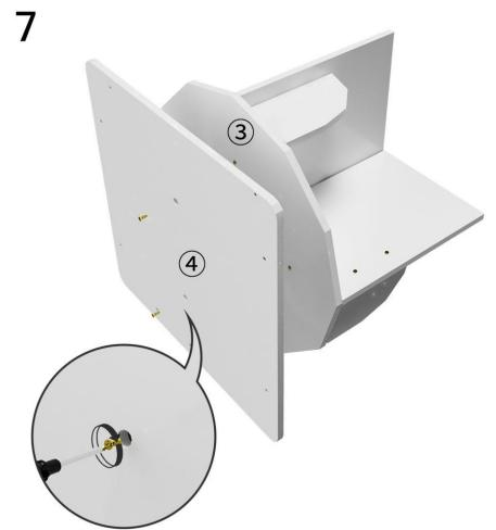
Reverse the ④ bottom board, Align the ③ ④ two boards
