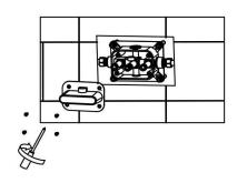
10. Insert the parts of shower head into the pre-embedded main body according to the corresponding hole.
