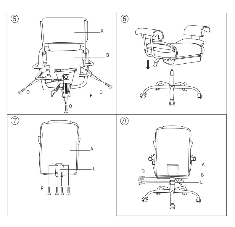
Please follow steps 5 to 8 to install the armrests and footrest on the seat. Then assembled the base, the backrest and the seat.
