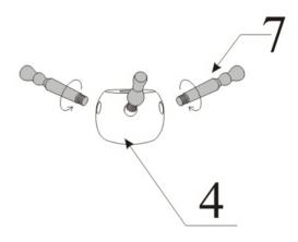
Firstly, screw the suspension bracket (7) into the support pillar (6) according to the angle
