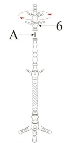
Finally, install the short screw and tighten (6) securely, completing the installation
