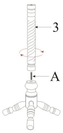
Screw screw A into the (2) pillar for 3-4 turns, then screw (3) in and fix it securely
