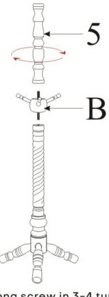
Screw the long screw in 3-4 turns, then fit the spherical body onto it, and finally screw in (5) to install and fix it securely
