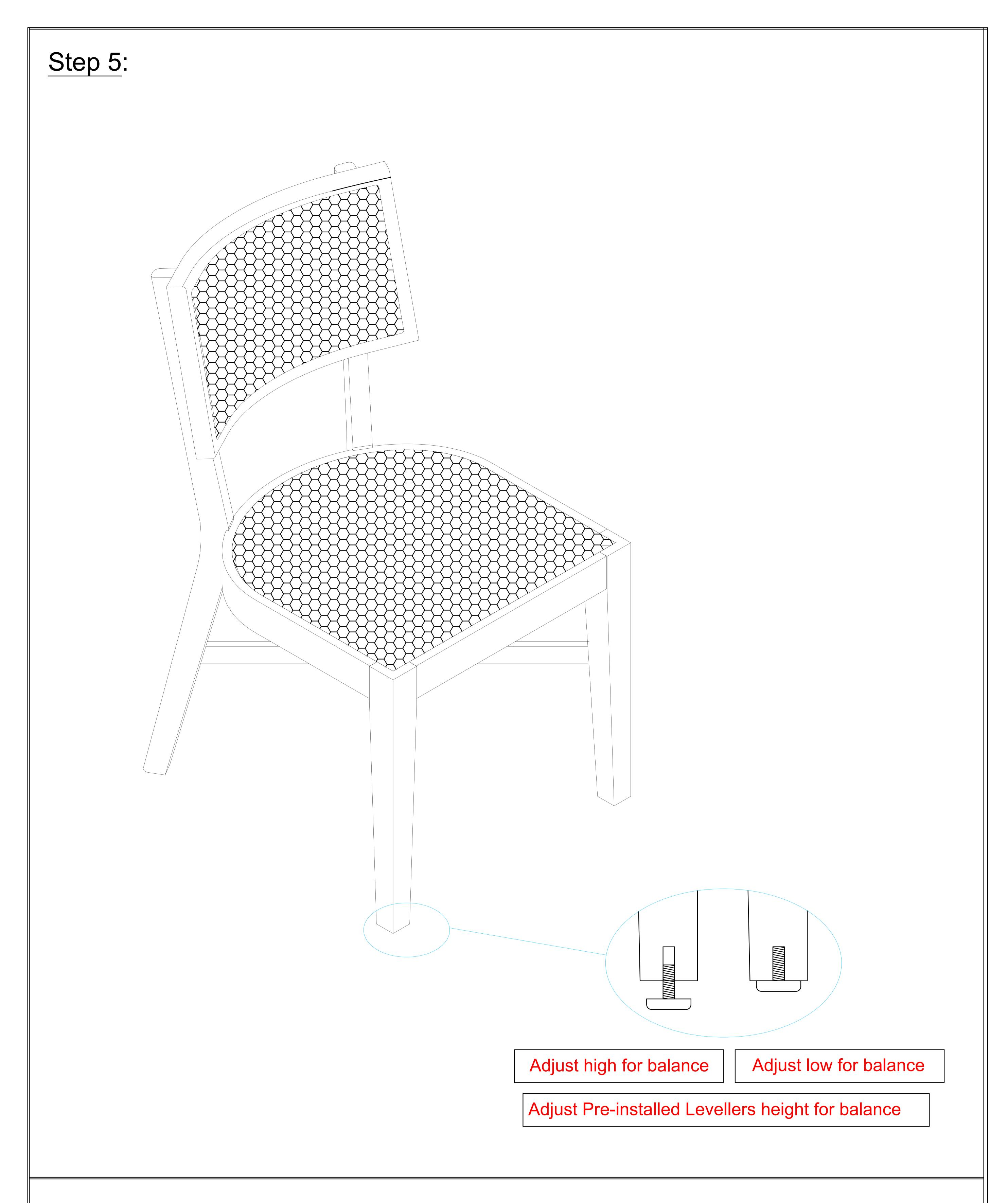
Inspect it and make sure all parts are adequately connected.
