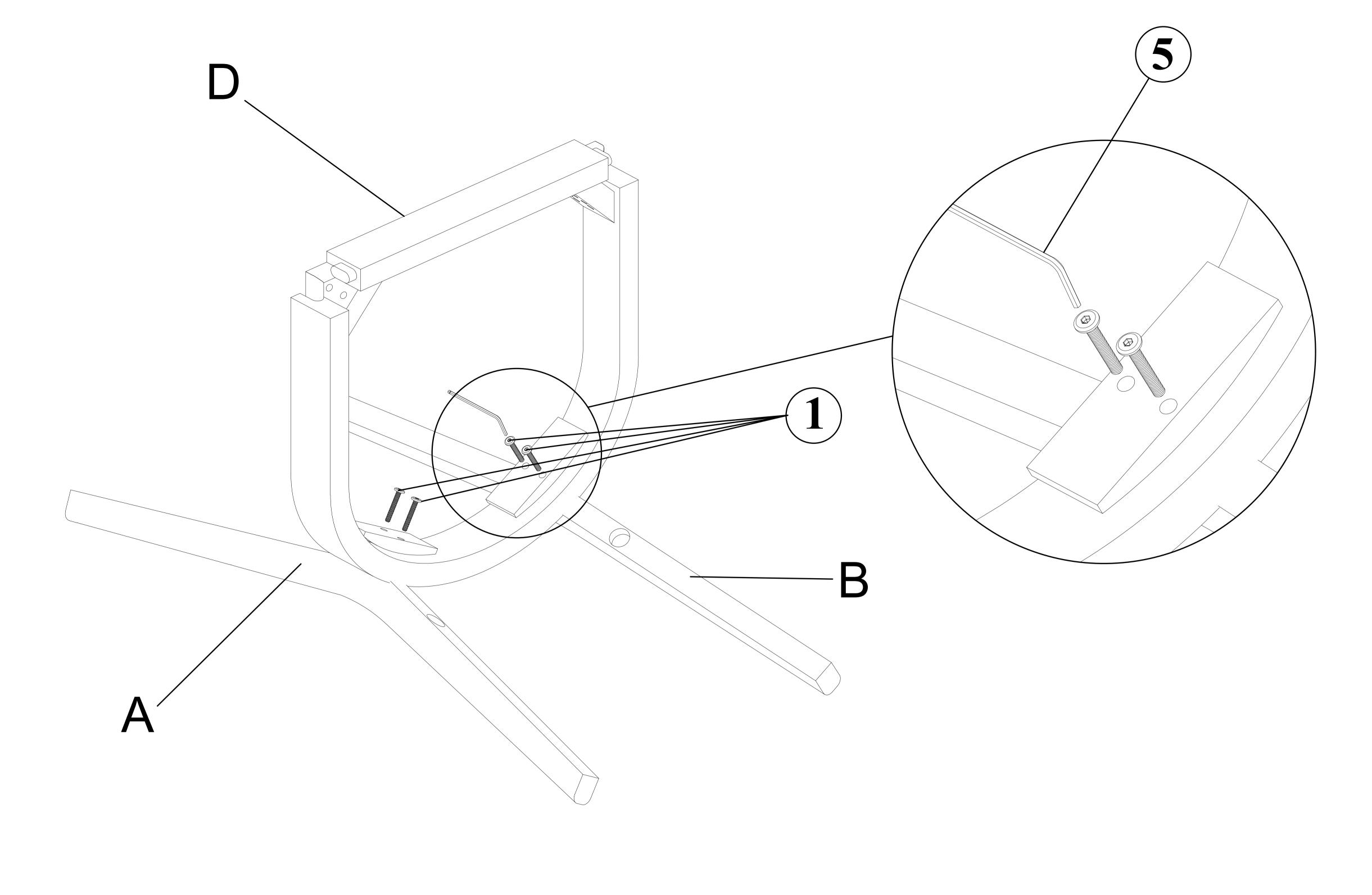
Fix the Left Back Leg (A) and Right Back Leg (B) with the Seat Panel (D) by using 4pcs Bolts (1) by Allen Wrench (5).
