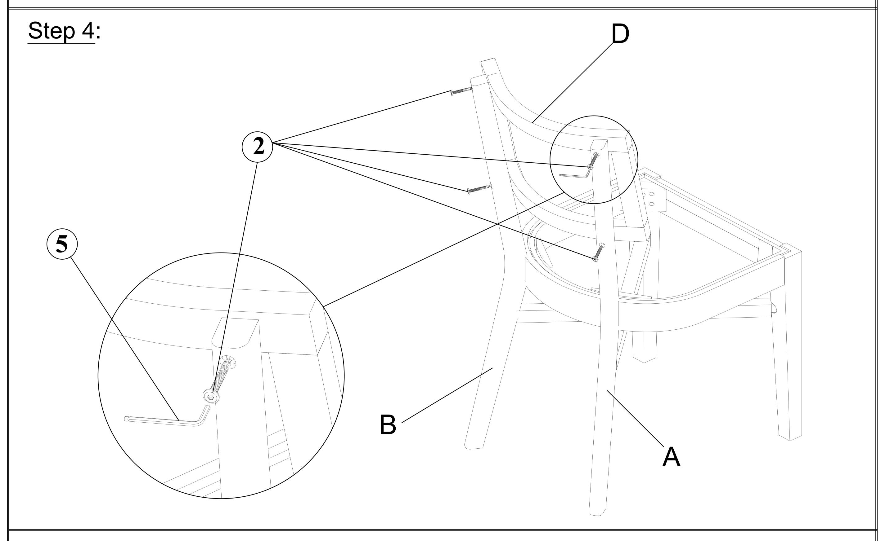
With the help of your adult partner, stand up the assembled parts in Step 3, place the Backrest (D) and then secure by using 4pcs Screws (2) and Allen Wrench (5) as shown above. **DO NOT fully tighten the screws**.
