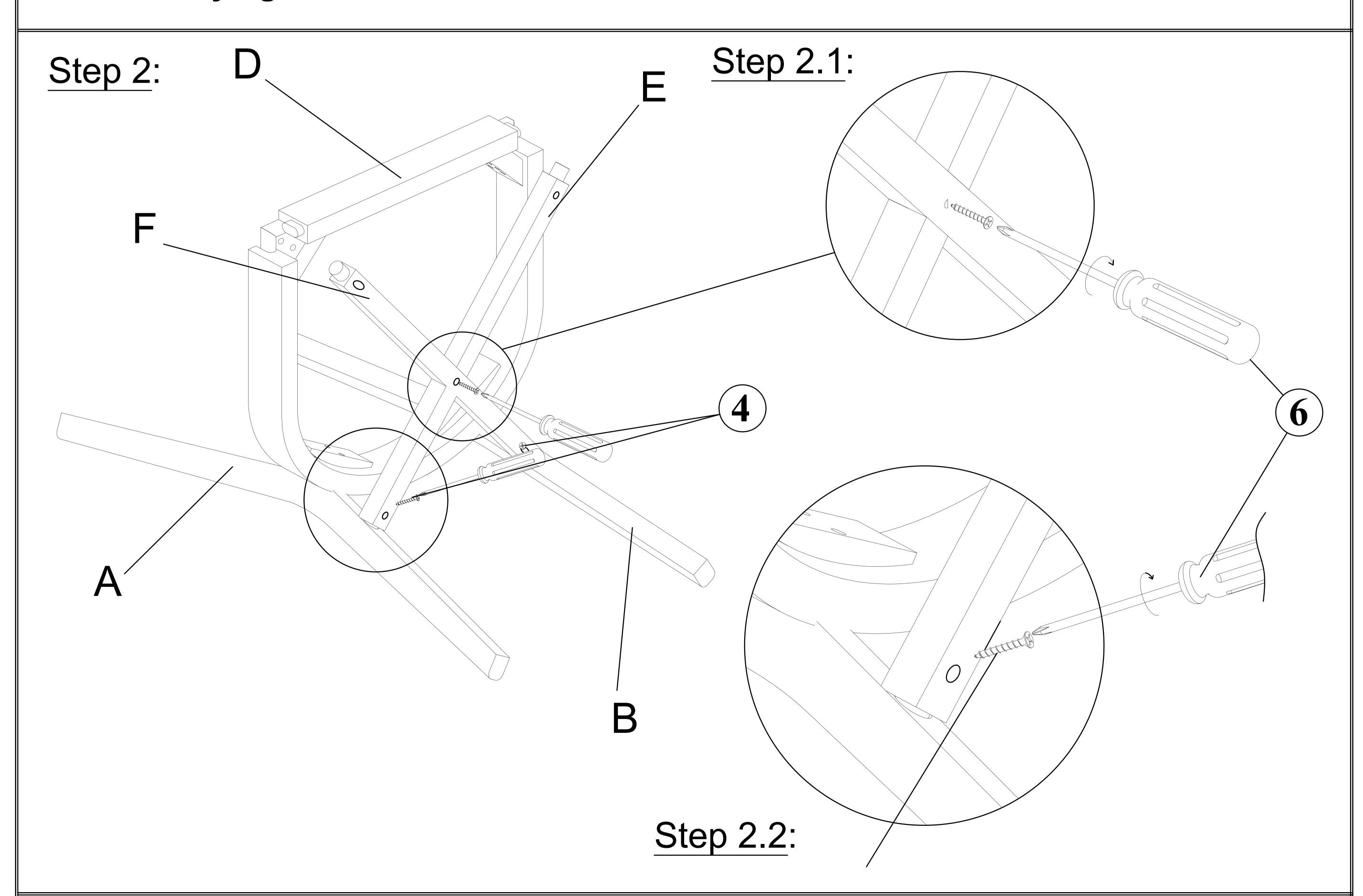
Fix the X-Support Bar (E) with Left Back Leg (A) and Right Back Leg(B) by using 2pcs Screws (4) by Allen Wrench (5).
