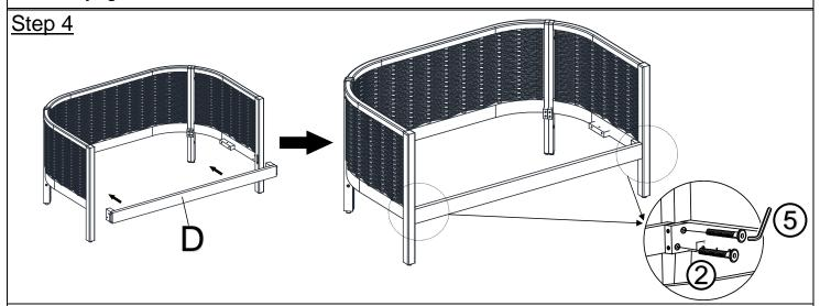
With assistance from your adult partner(s), attach the Support Bar (D) to the assembled frame in step 3 by using Bolts (2) and the Allen Wrench (5) as shown above.
