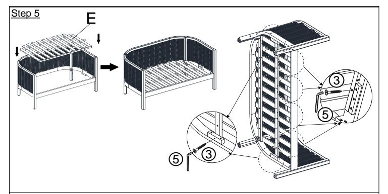
With assistance from your adult partner(s), attach the Seat Panel (E) into the assembled parts in step 4 using Screws ( $\Im$ ) and the Allen Wrench ( $\Im$ ) as shown in the above picture.
